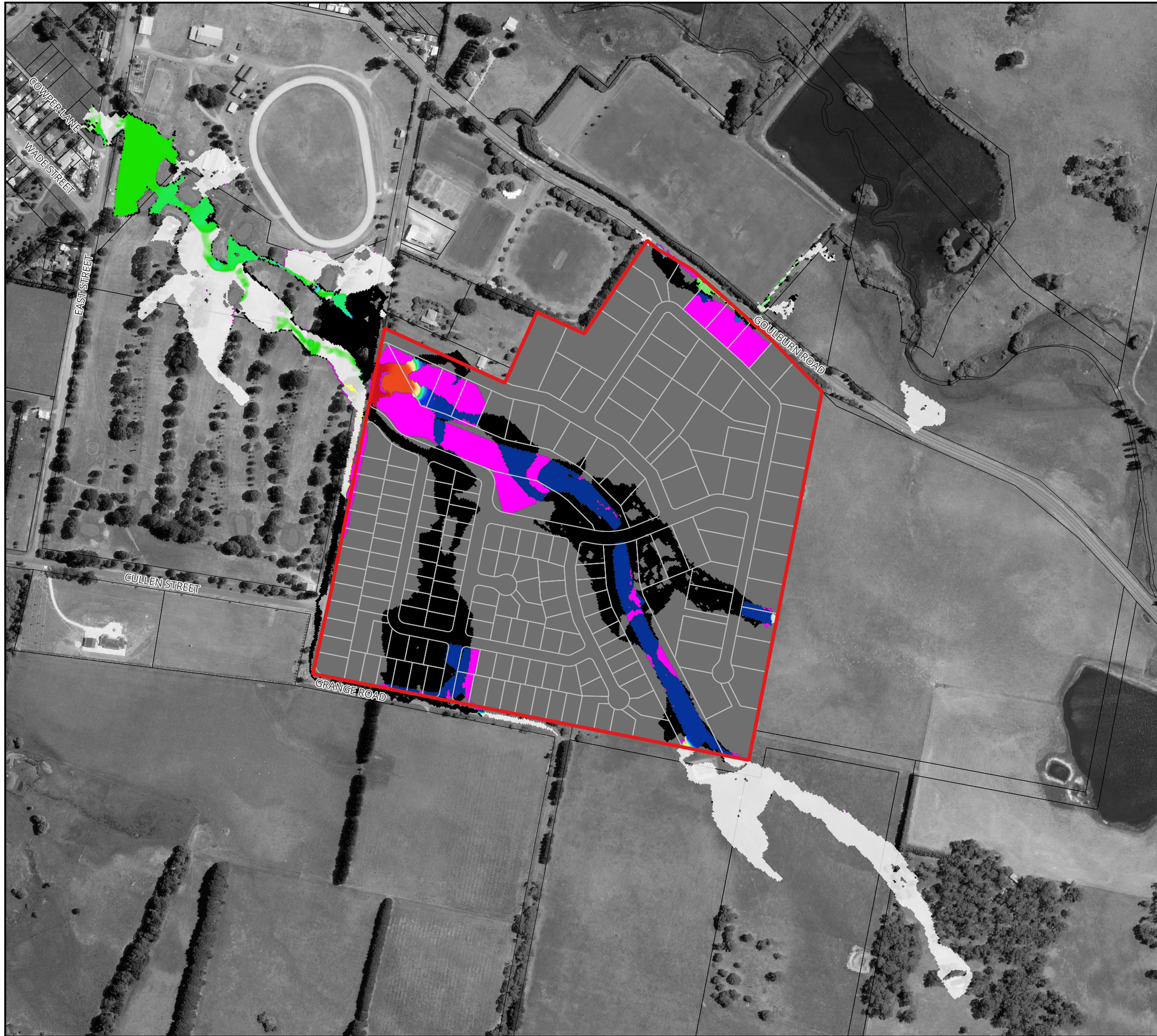
Figure 70 : Predicted Change in Peak 50% AEP Flood Levels
