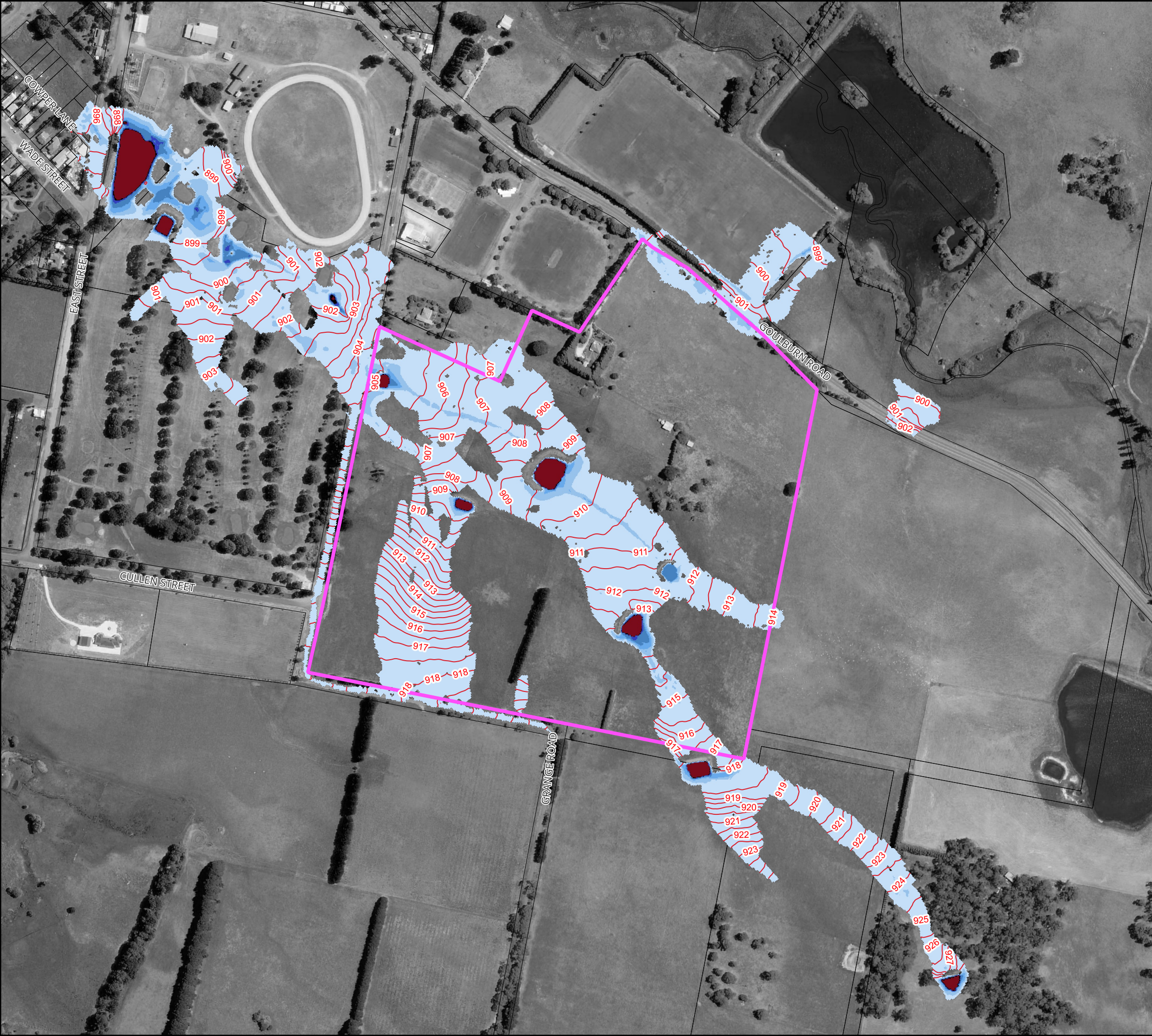
Figure 11 : Peak Floodwater Depths and Levels for the 0.5% AEP Flood for Existing Conditions
