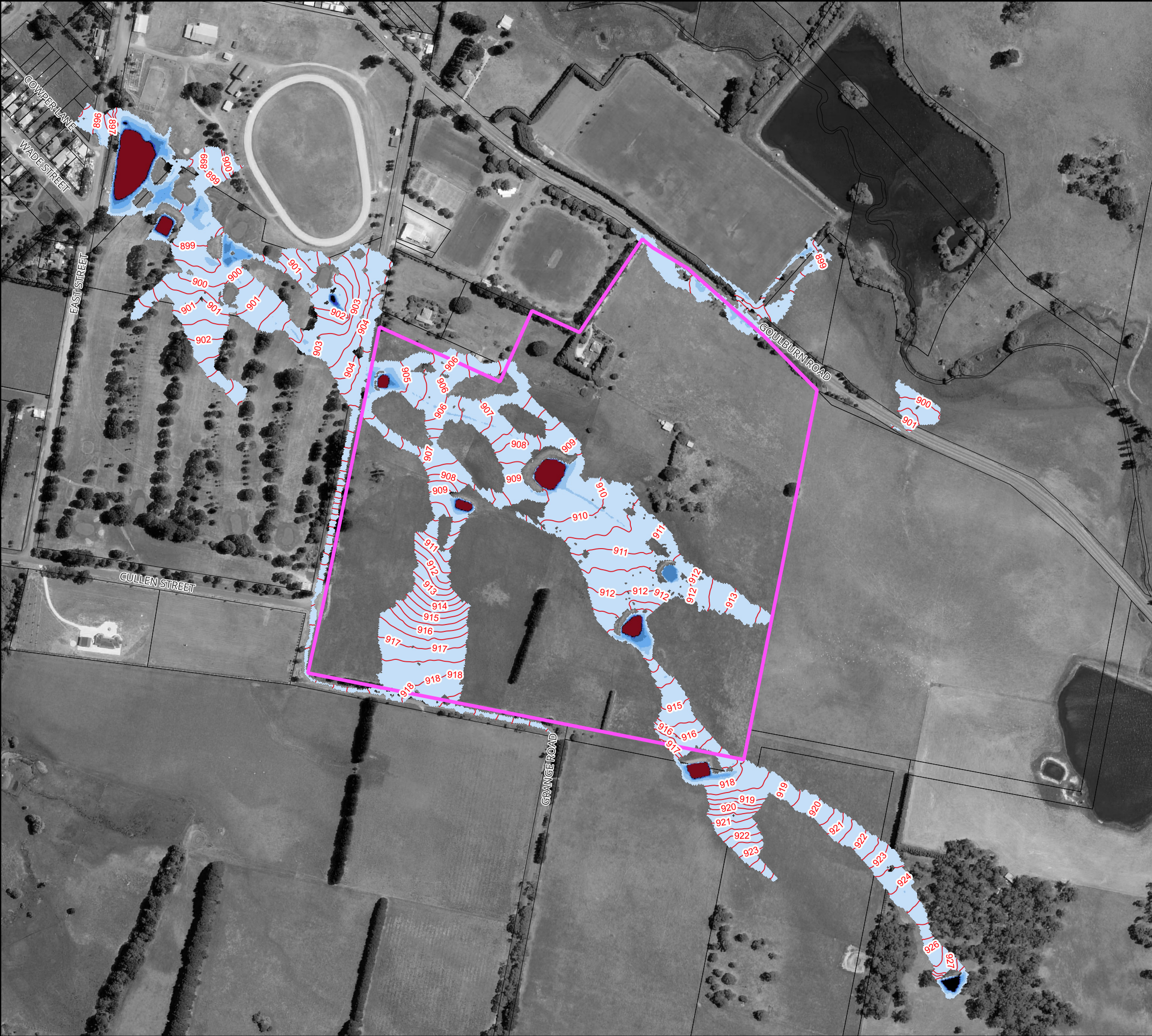
Figure 6 : Peak Floodwater Depths and Levels for the 20% AEP Flood for Existing Conditions
