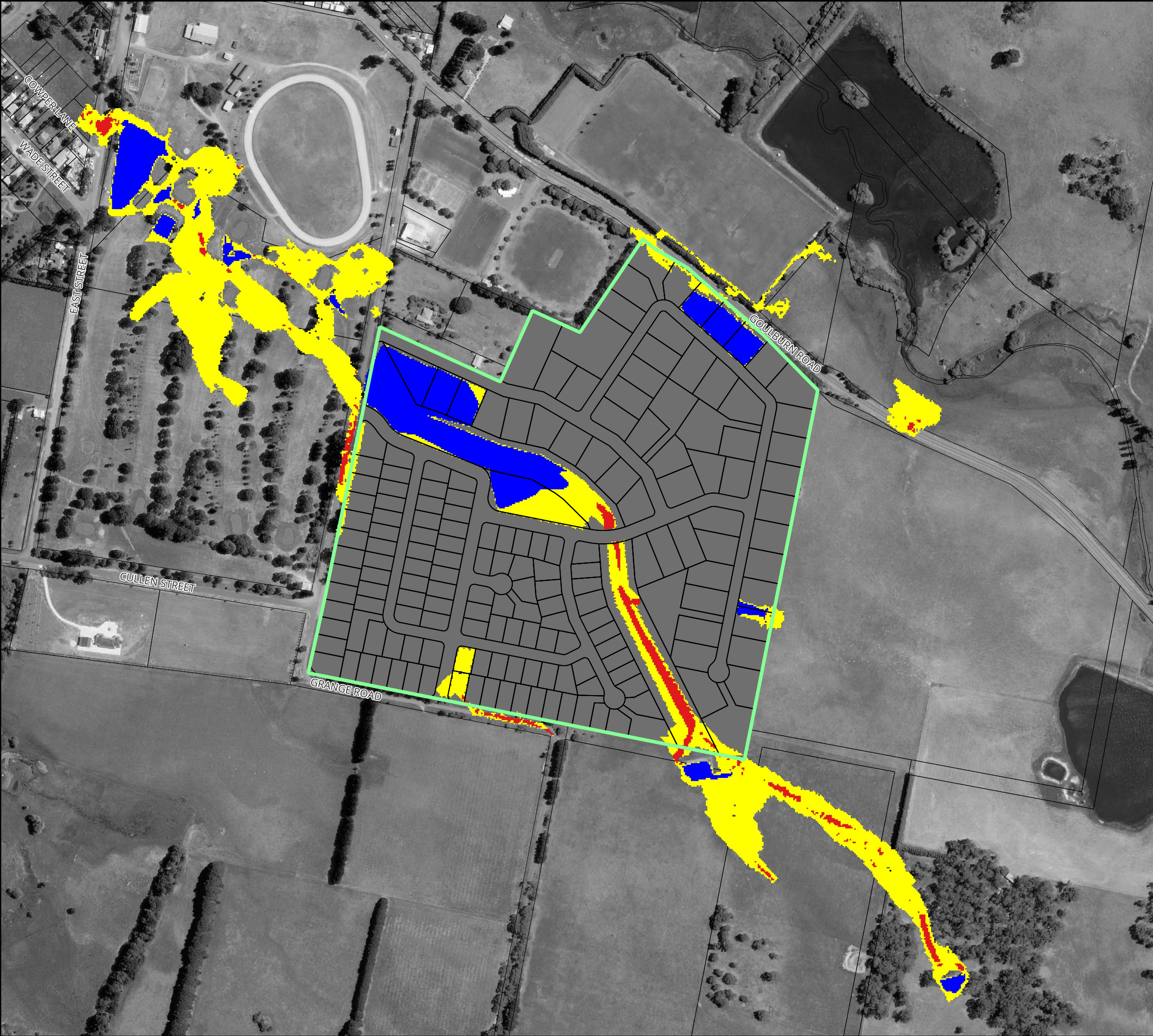
Figure 57 : Hydraulic Categories for the 1% AEP Flood for Proposed Conditions
