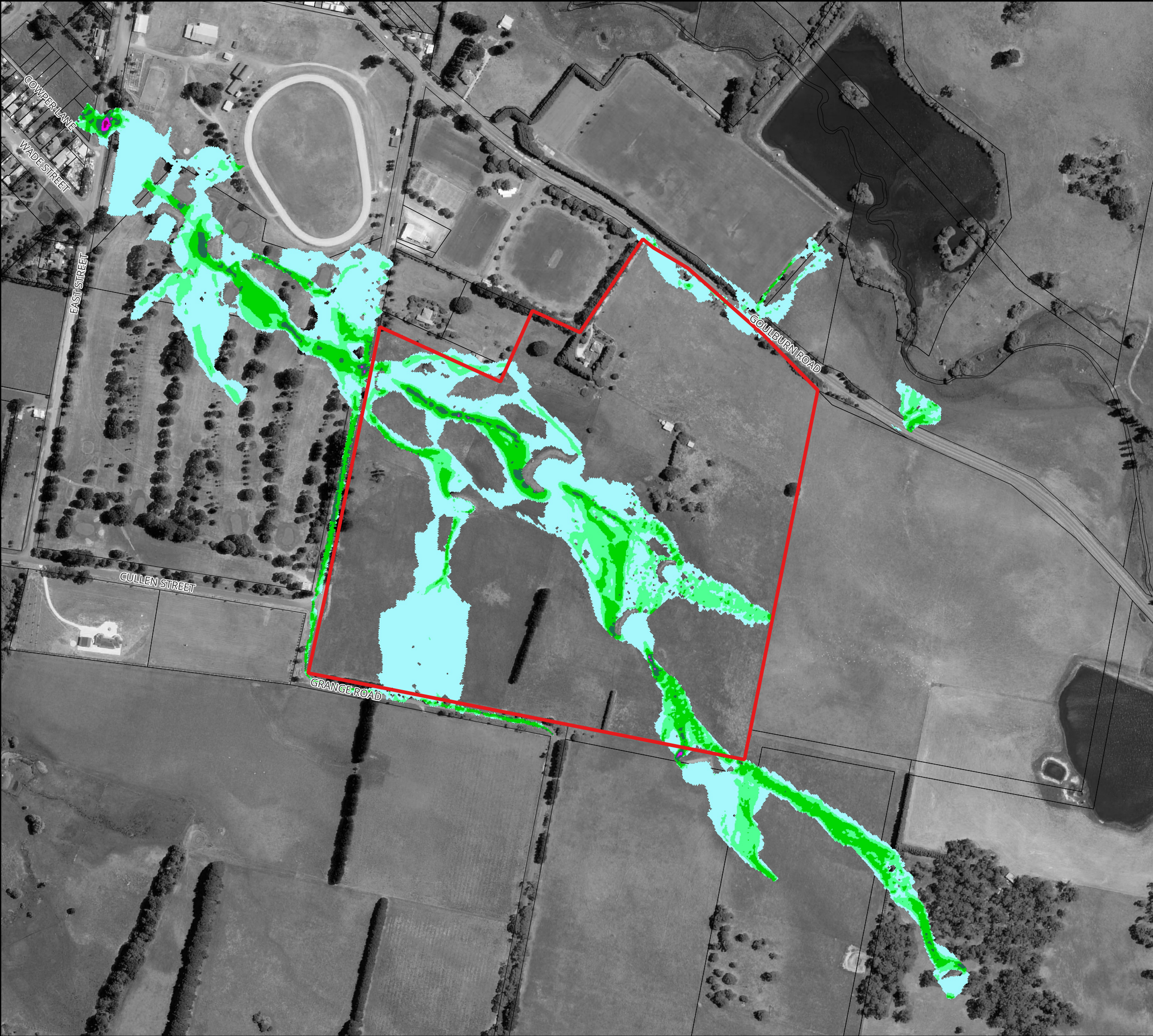
Figure 16 : Peak Flood Velocity for the 20% AEP Flood for Existing Conditions
