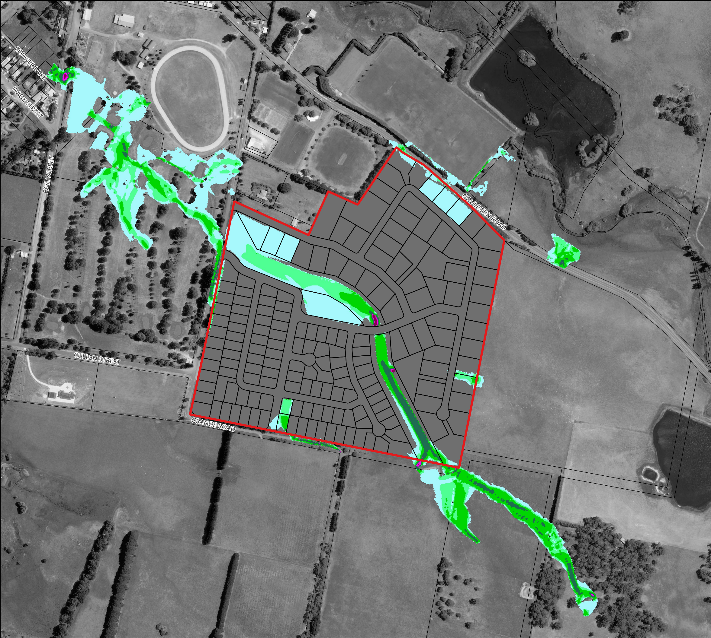
Figure 54 : Peak Flood Velocity for the 0.5% AEP Flood for Proposed Conditions
