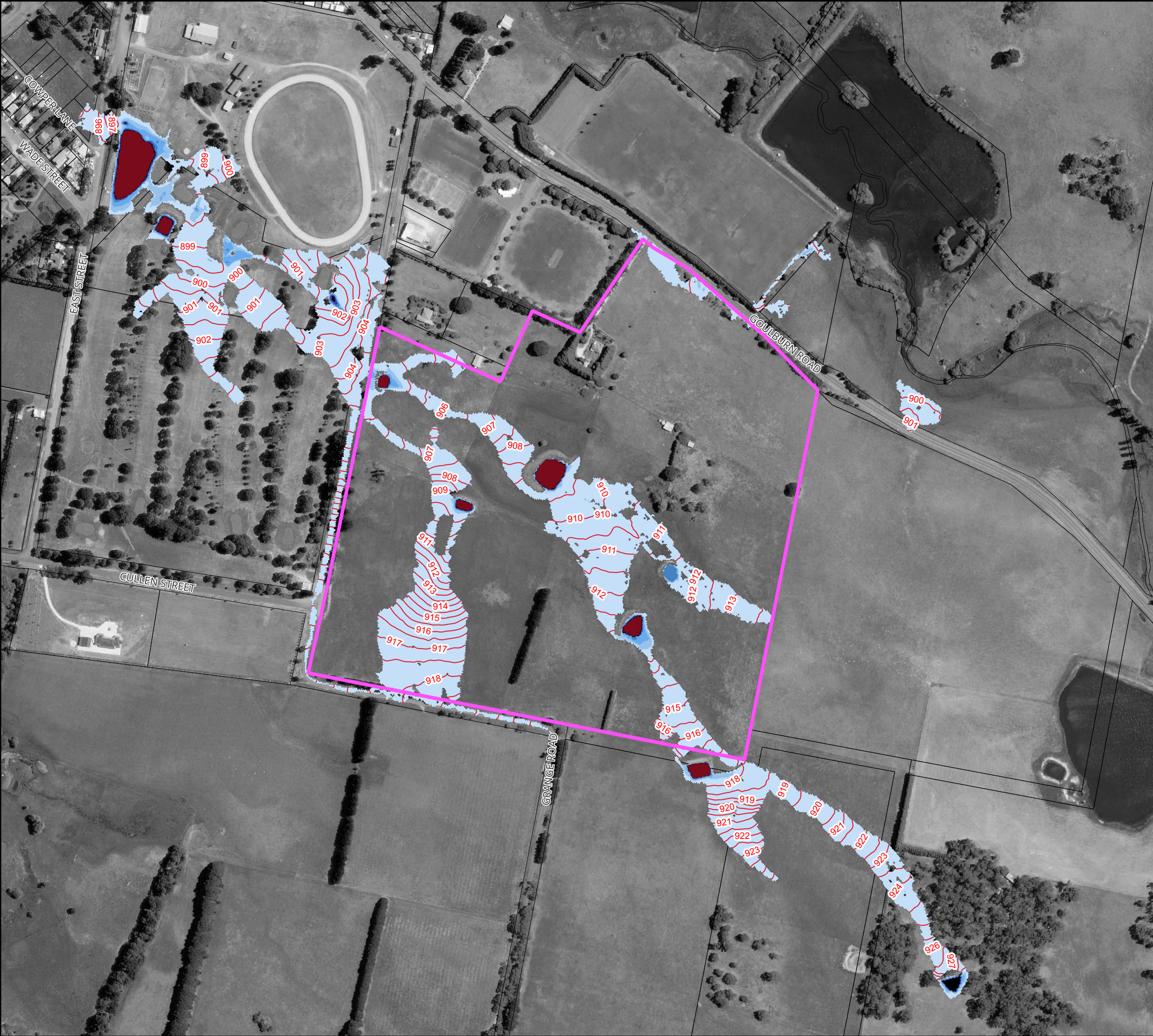
Figure 4 : Peak Floodwater Depths and Levels for the 63.2% AEP Flood for Existing Conditions
