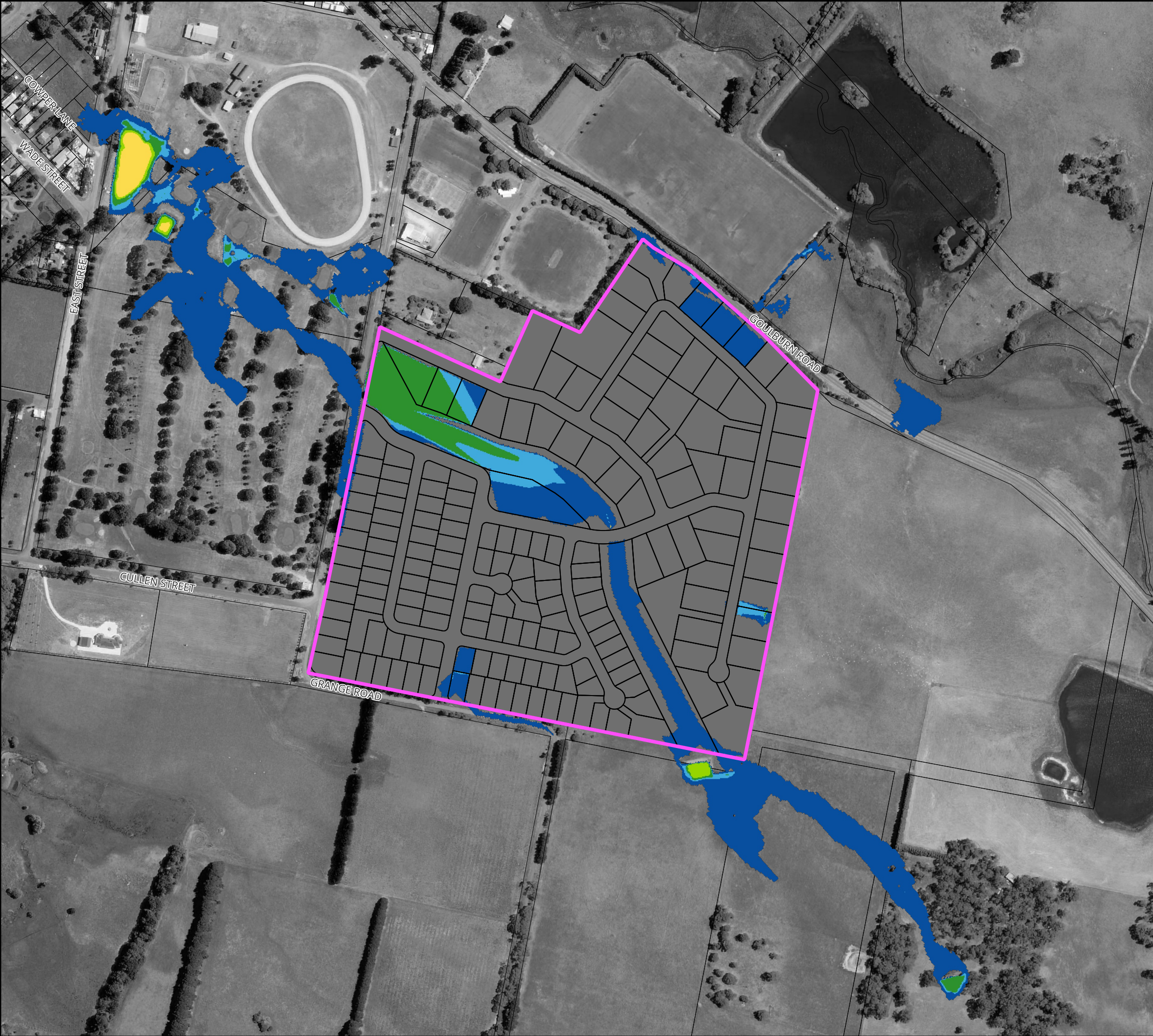
Figure 62 : Flood Hazard for the 10% AEP Flood for Proposed Conditions
