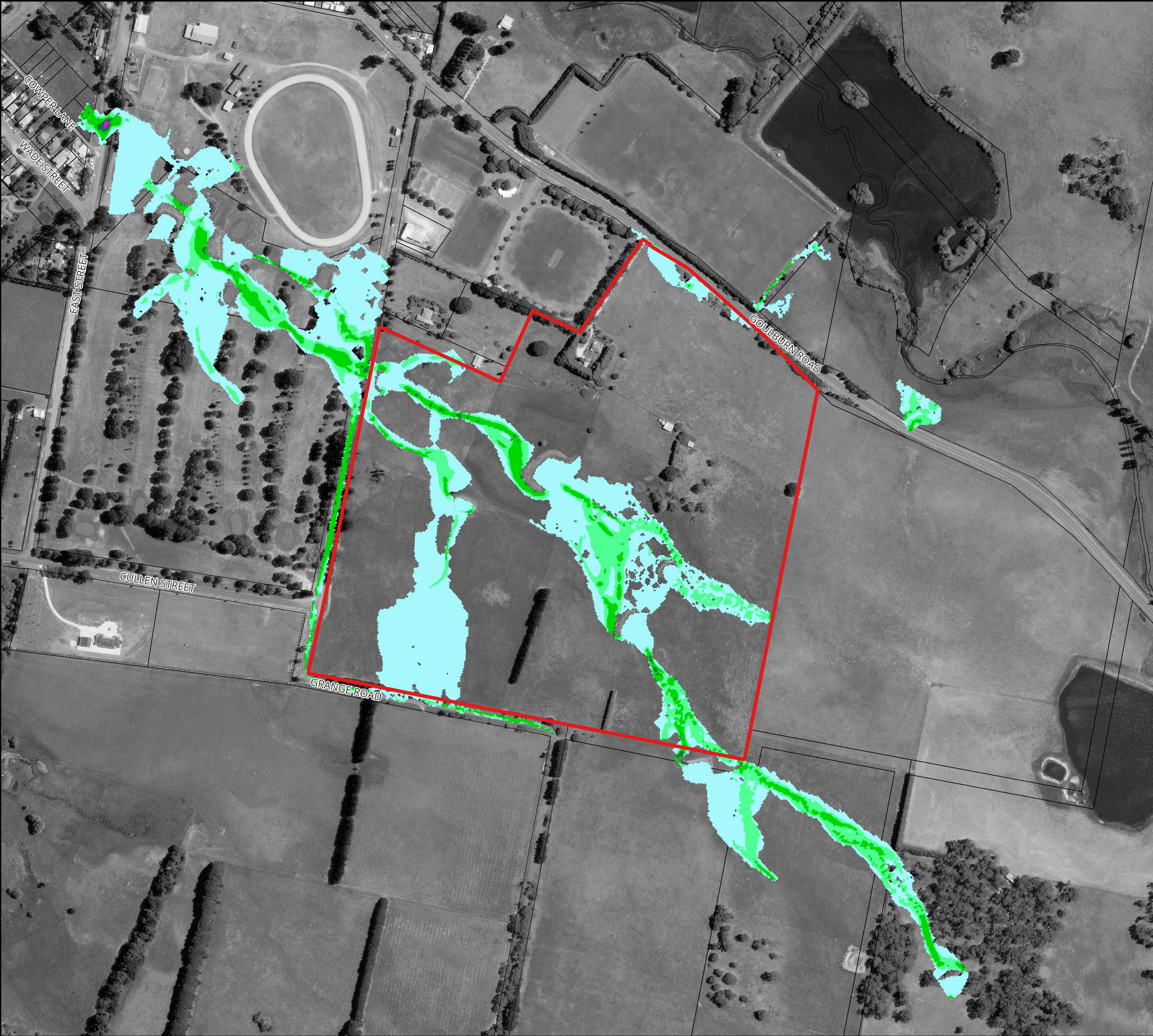
Figure 15 : Peak Flood Velocity for the 50% AEP Flood for Existing Conditions
