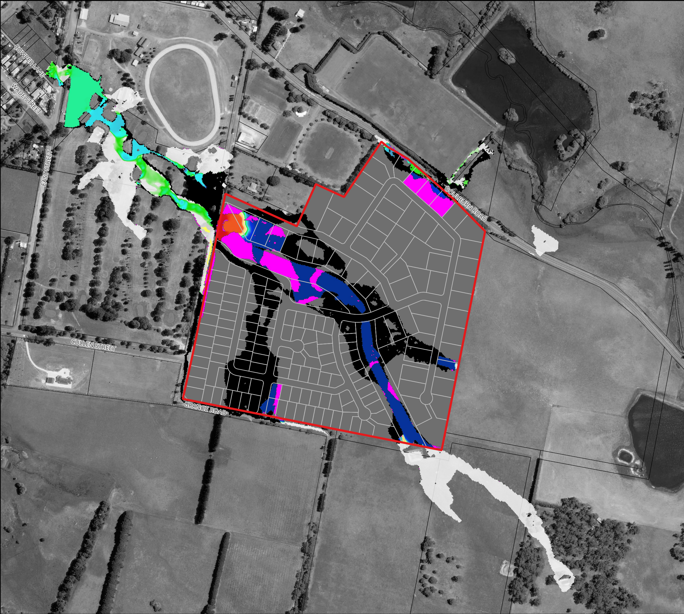
Figure 71 : Predicted Change in Peak 20% AEP Flood Levels
