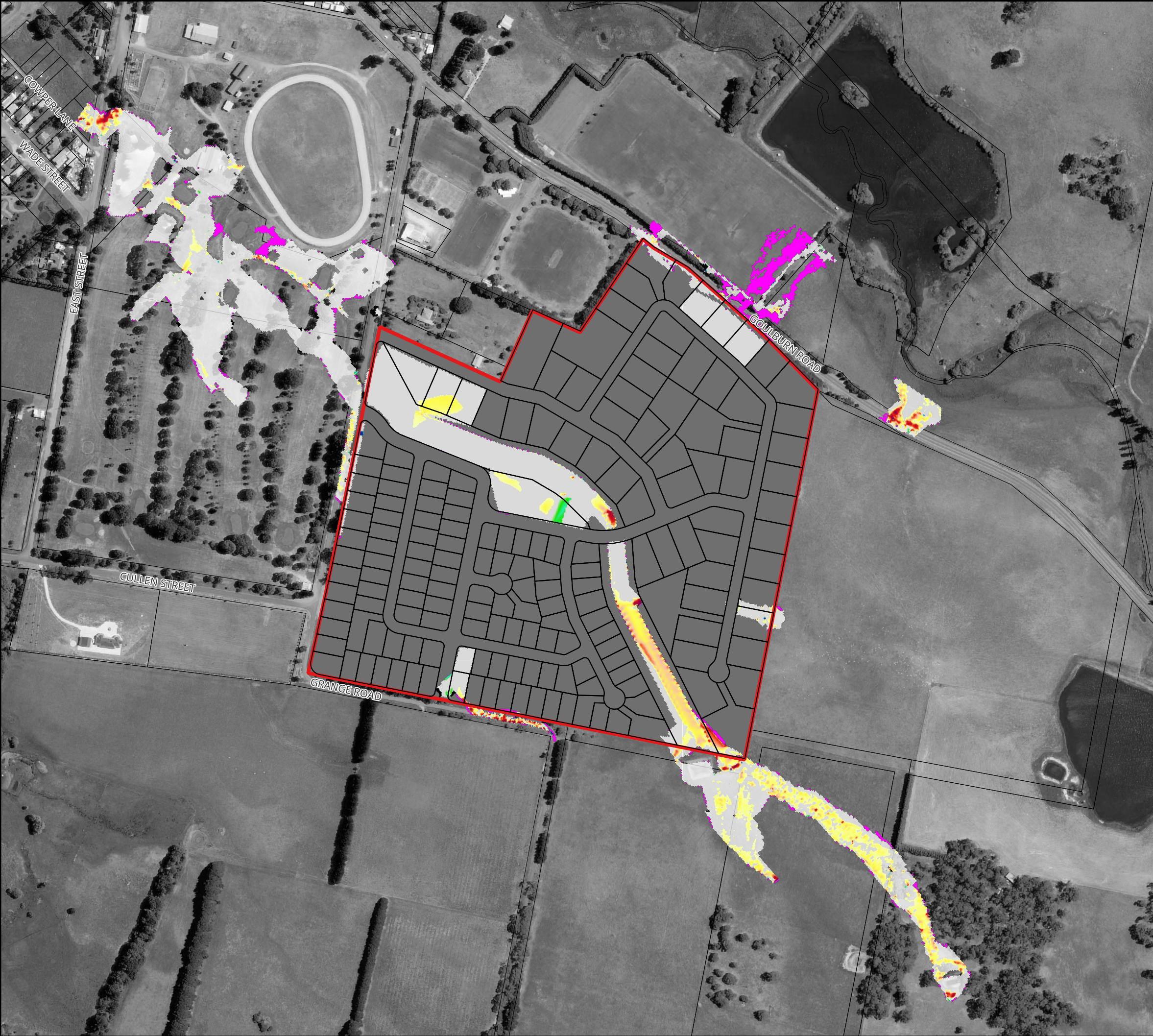
Figure 92 : Predicted Change in Peak 1% AEP Flood Velocity as a result of Climate Change using the 0.2% AEP Event as a Proxy
