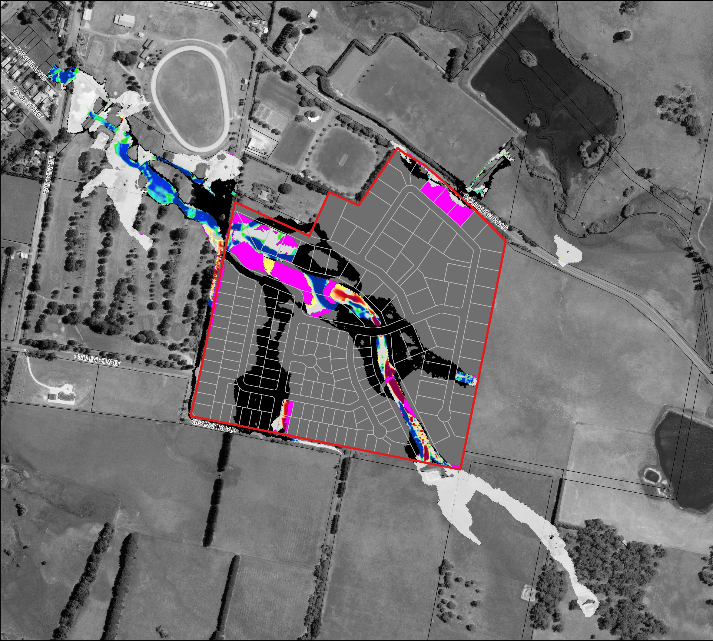
Figure 81 : Predicted Change in Peak 20% AEP Flood Velocity
