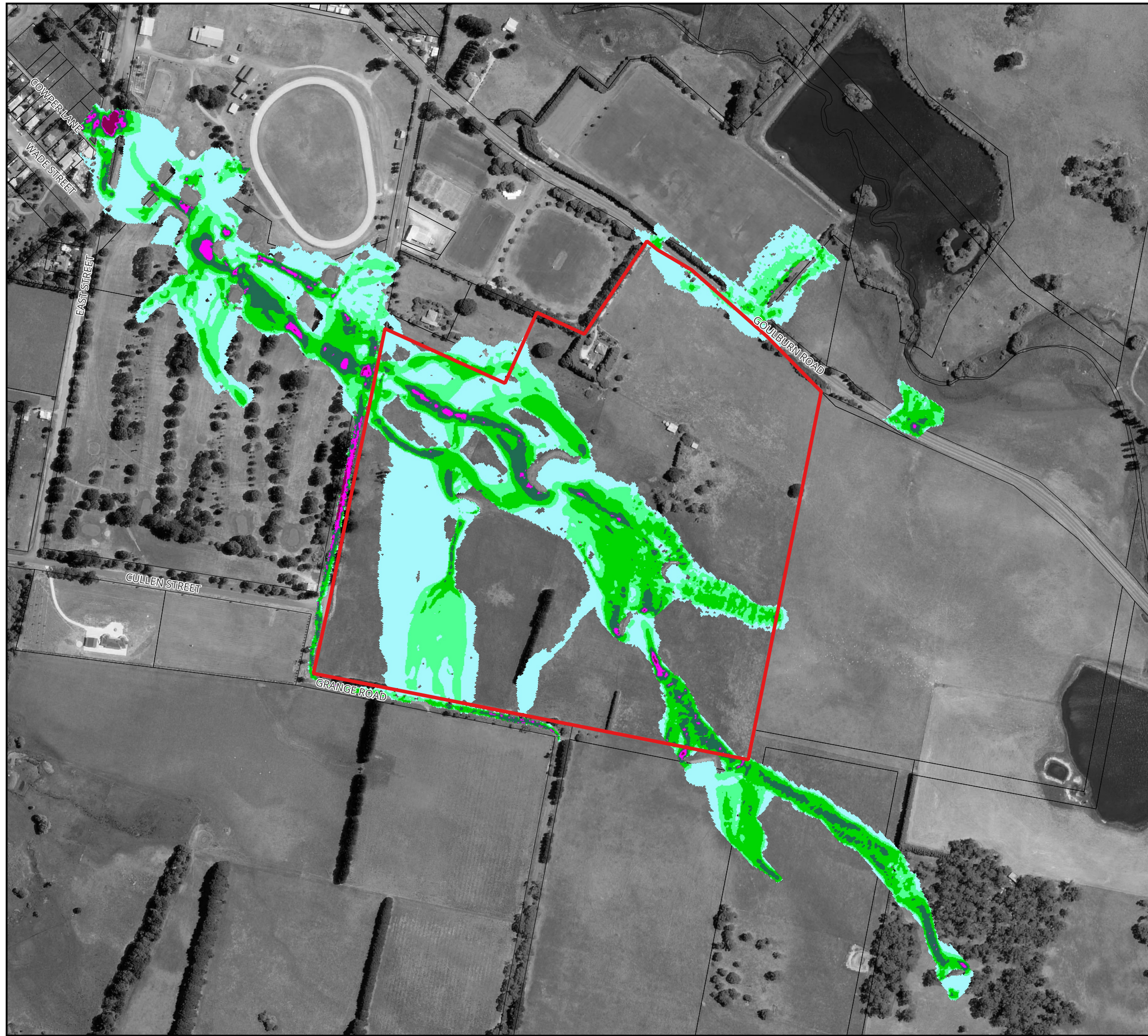
Figure 22 : Peak Flood Velocity for the 0.2% AEP Flood for Existing Conditions
