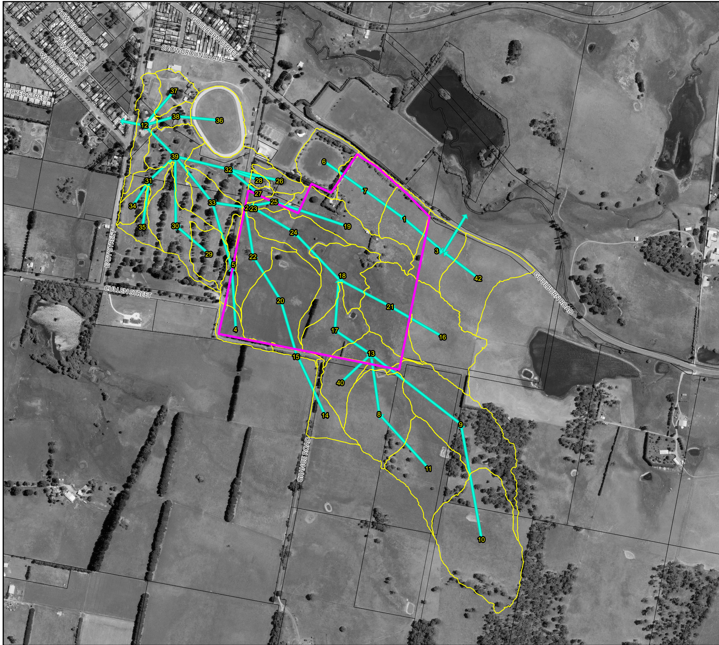
Figure 2 : XP-RAFTS Subcatchment Layout
