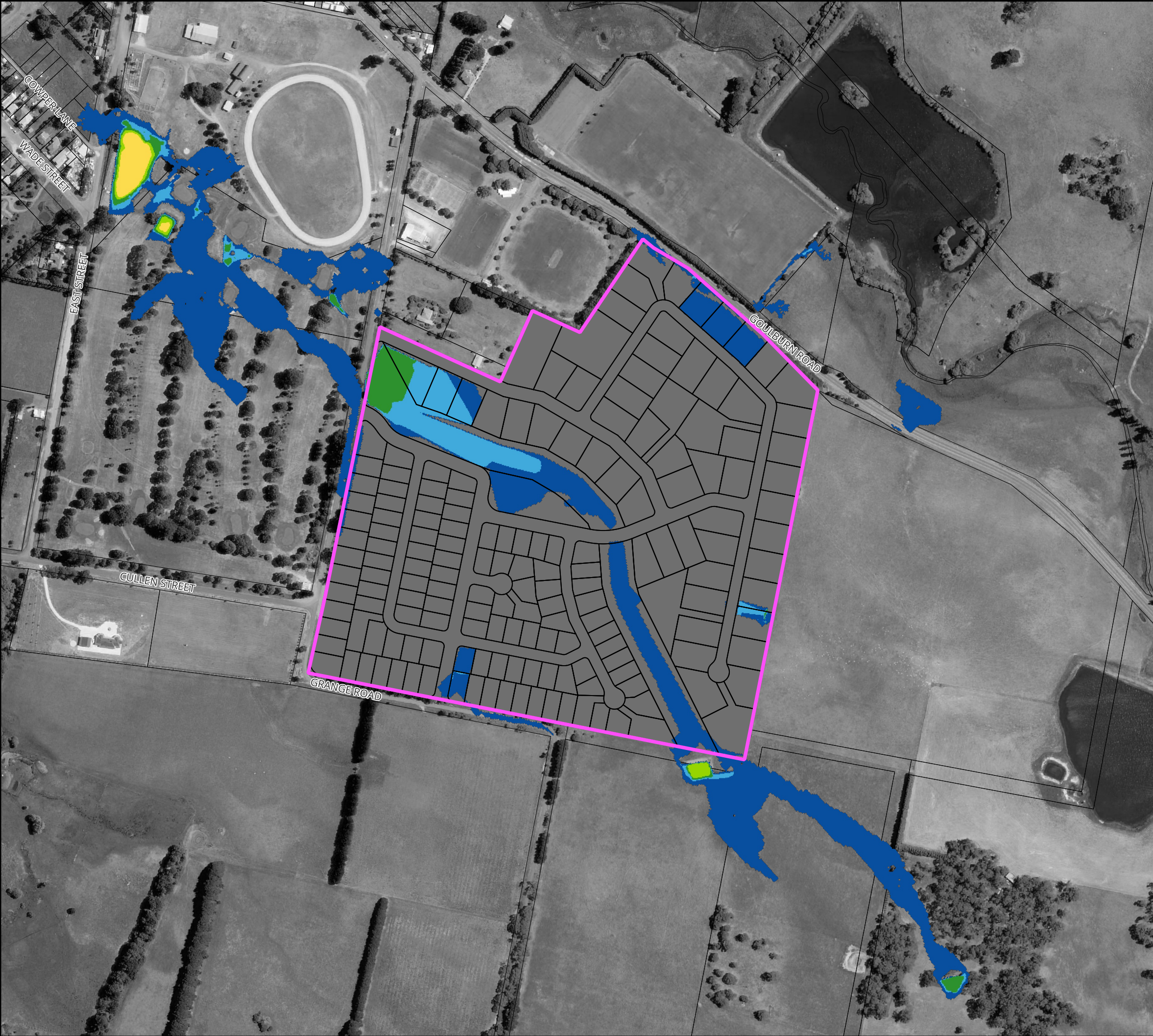
Figure 61 : Flood Hazard for the 20% AEP Flood for Proposed Conditions
