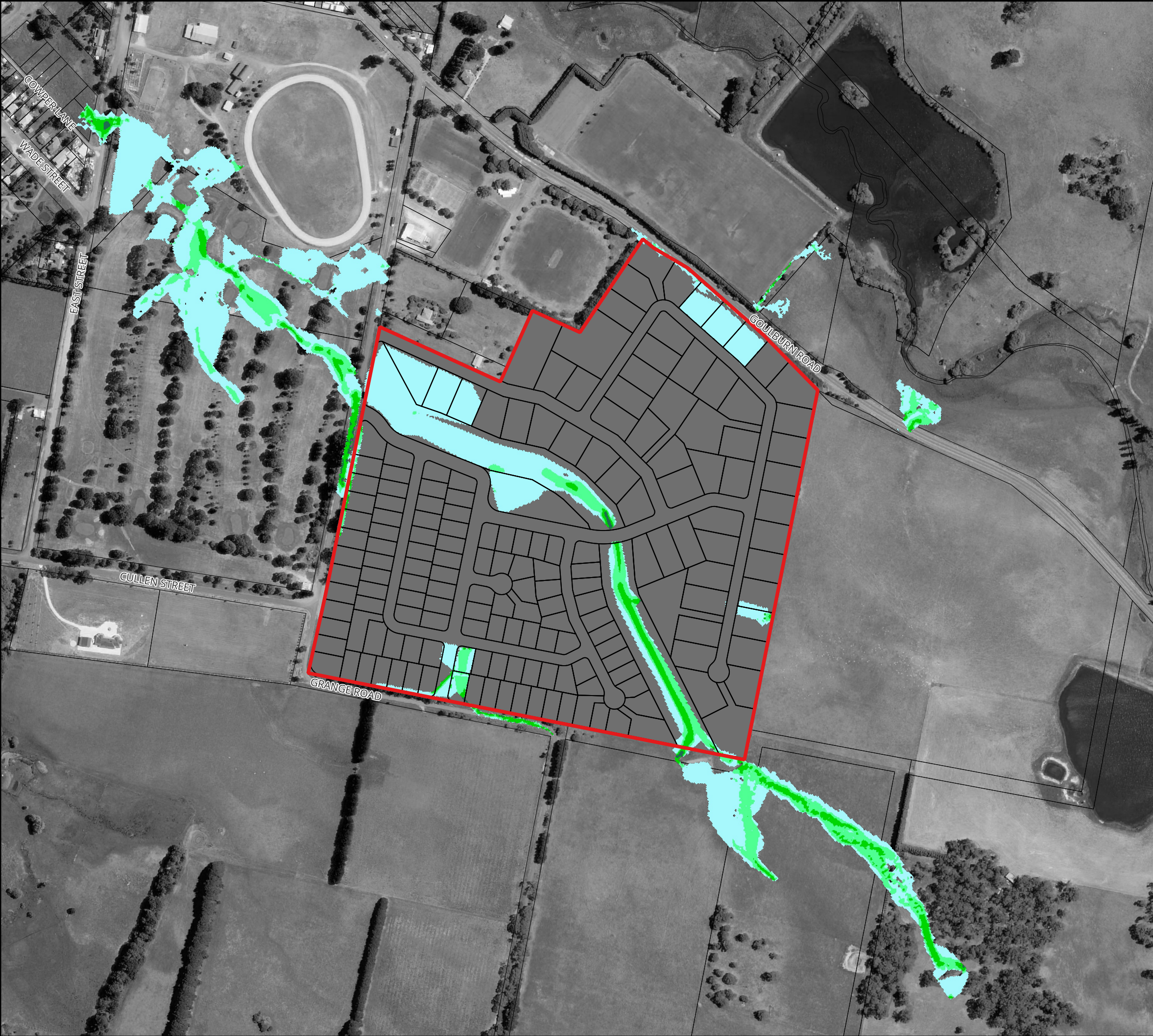
Figure 48 : Peak Flood Velocity for the 50% AEP Flood for Proposed Conditions
