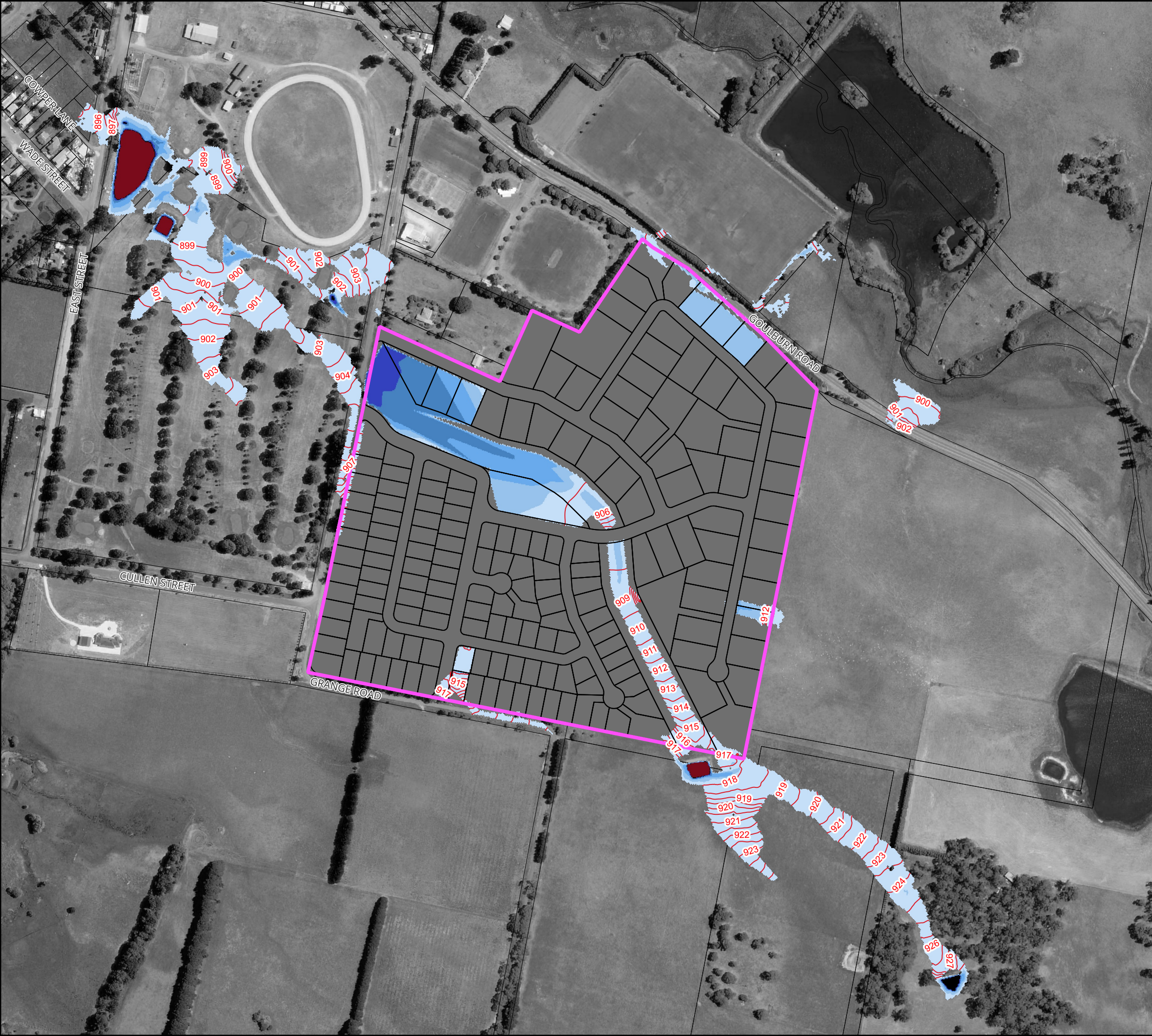
Figure 41 : Peak Floodwater Depths and Levels for the 5% AEP Flood for Proposed Conditions
