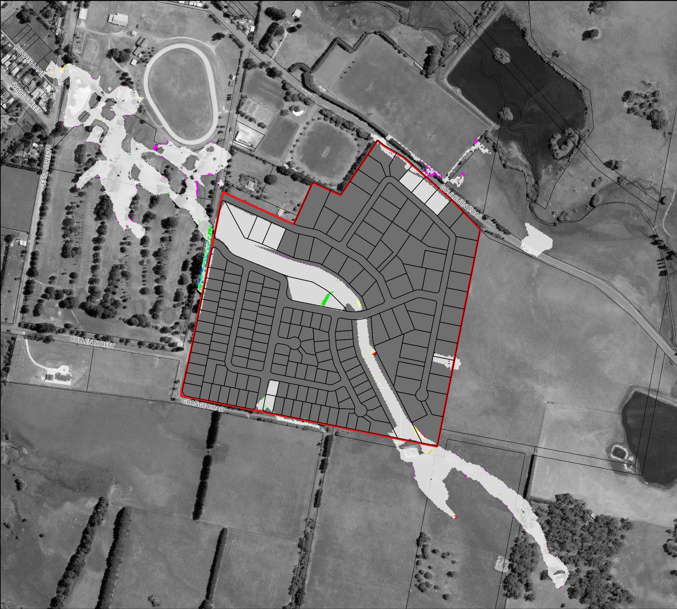
Figure 90 : Predicted Change in Peak 1% AEP Flood Velocity as a result of Climate Change using the 0.5% AEP Event as a Proxy
