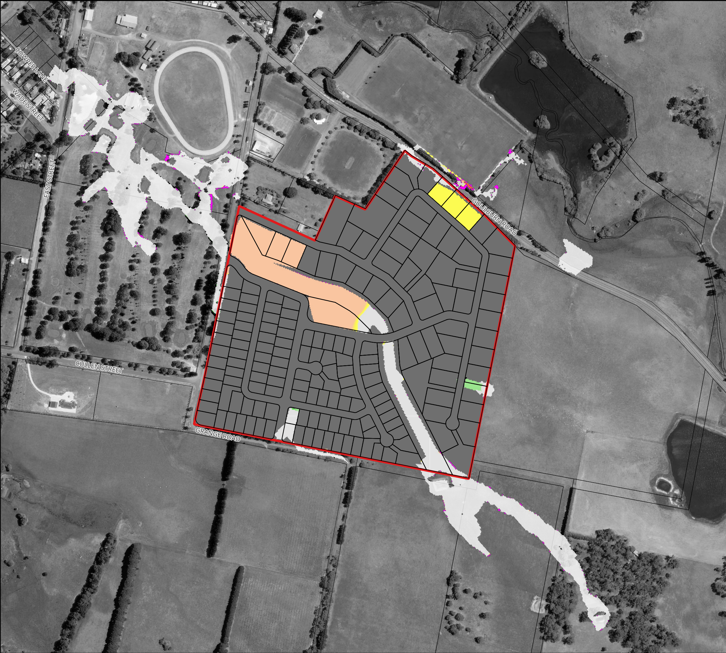
Figure 89 : Predicted Change in Peak 1% AEP Flood Levels as a result of Climate Change using the 0.5% AEP Event as a Proxy
