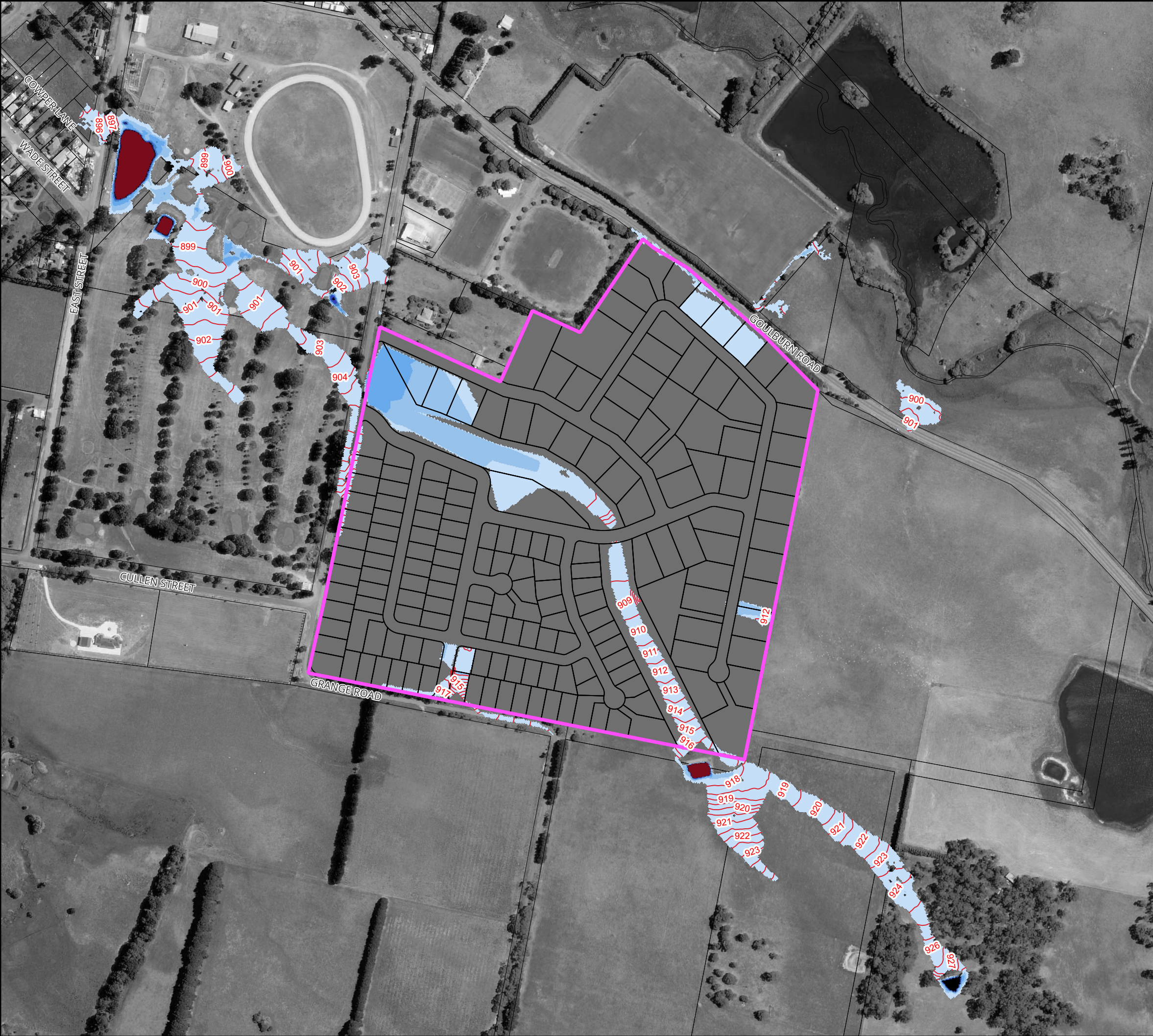
Figure 37 : Peak Floodwater Depths and Levels for the 63.2% AEP Flood for Proposed Conditions
