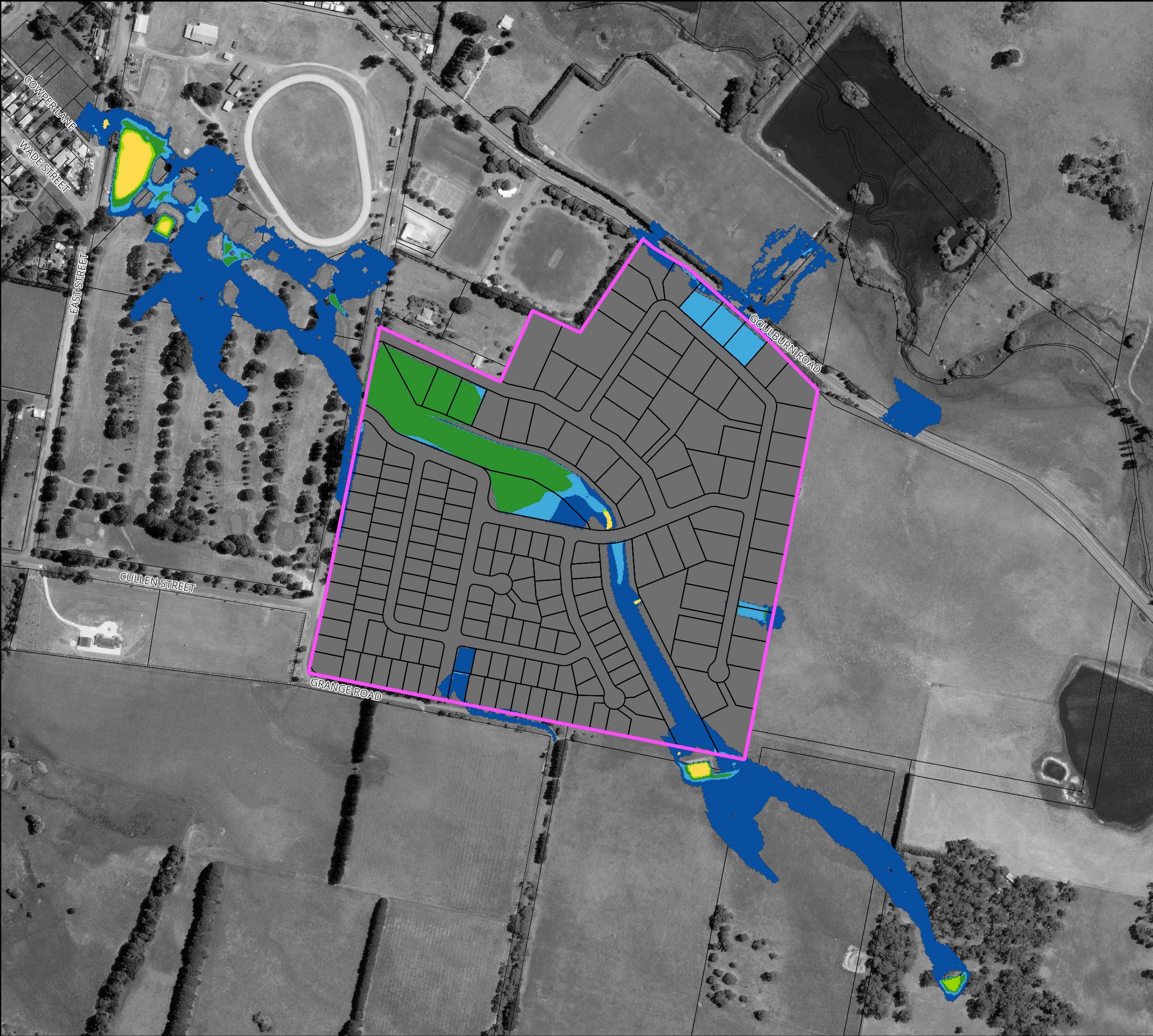
Figure 67 : Flood Hazard for the 0.2% AEP Flood for Proposed Conditions
