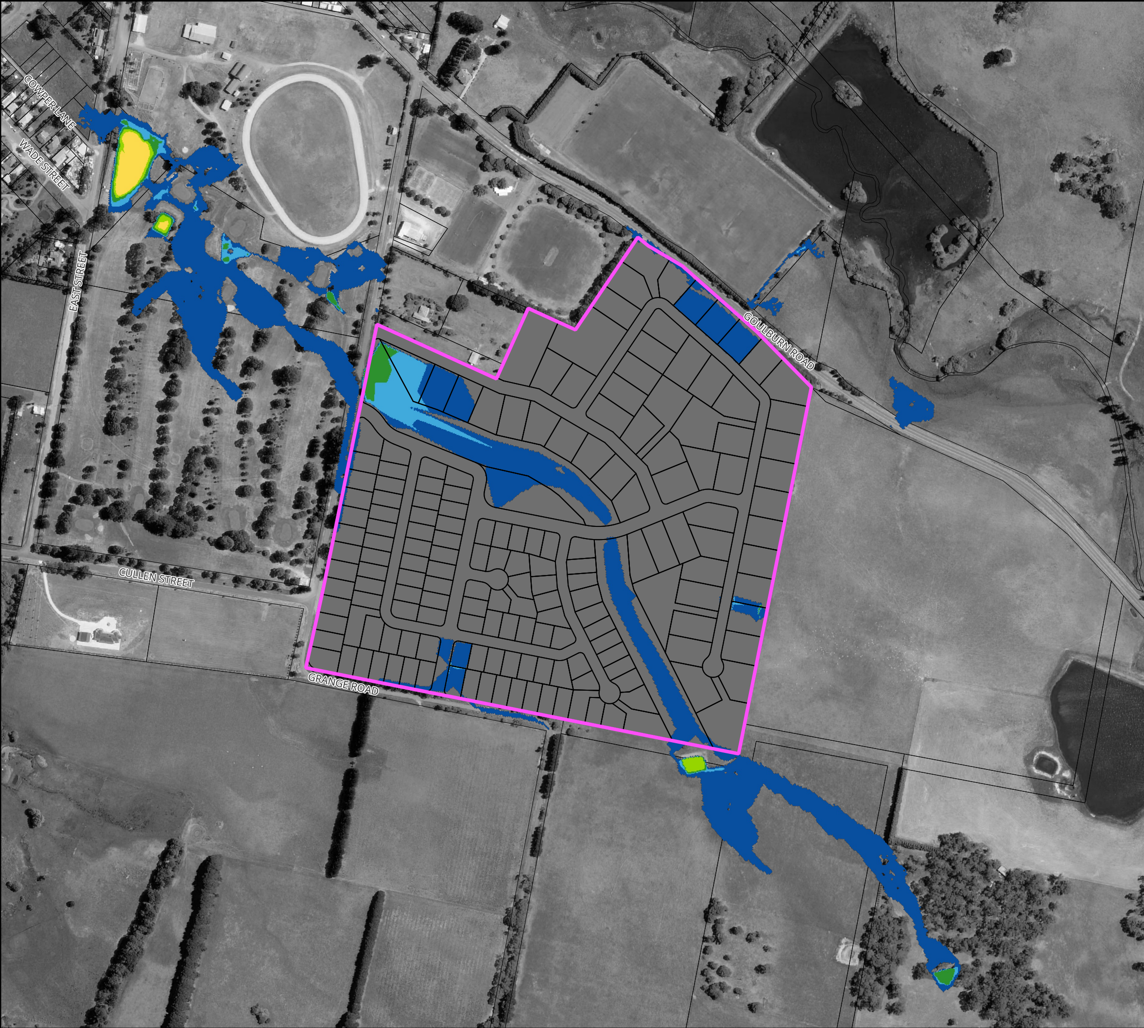
Figure 59 : Flood Hazard for the 63.2% AEP Flood for Proposed Conditions
