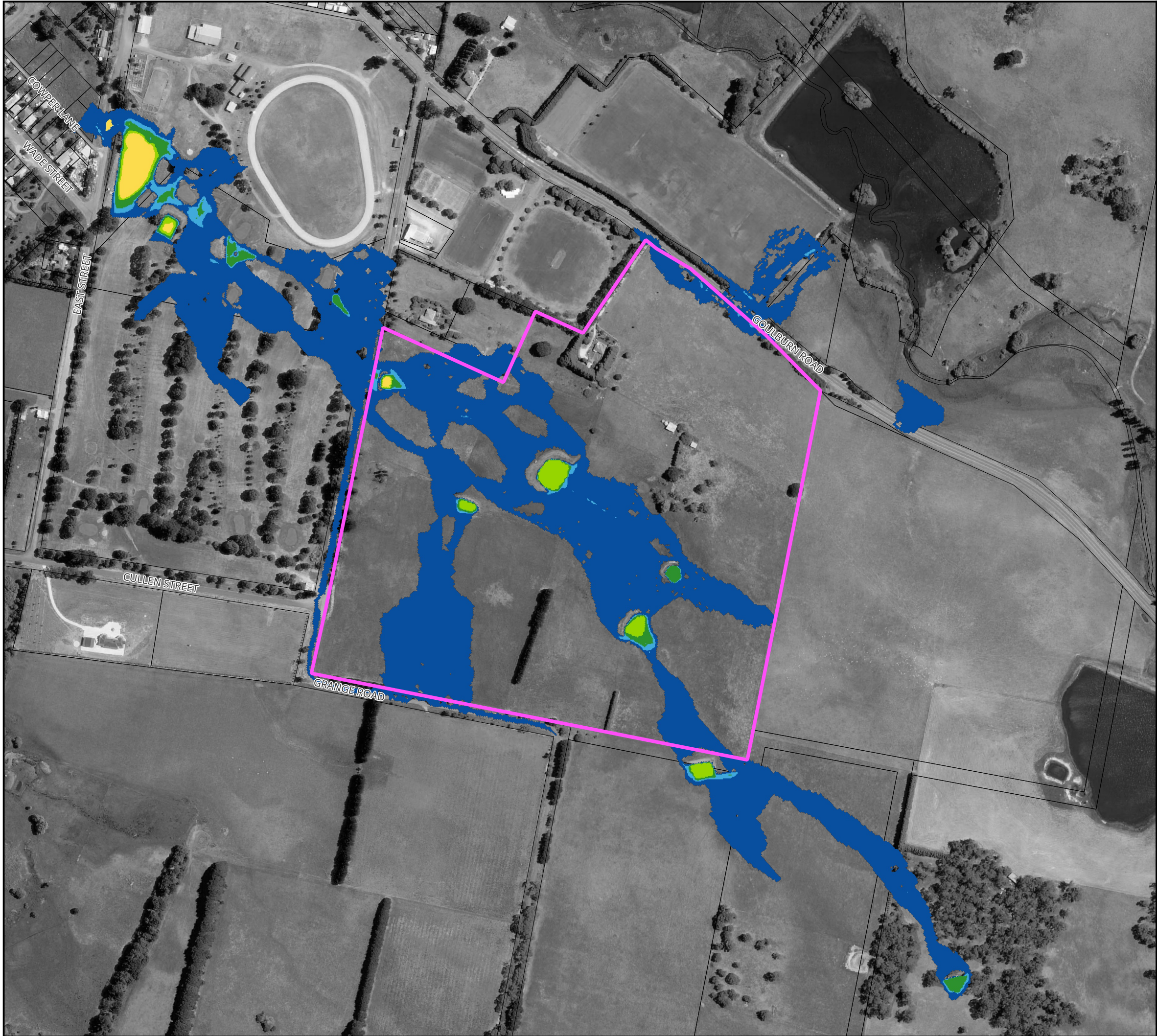
Figure 29 : Flood Hazard for the 10% AEP Flood for Existing Conditions
