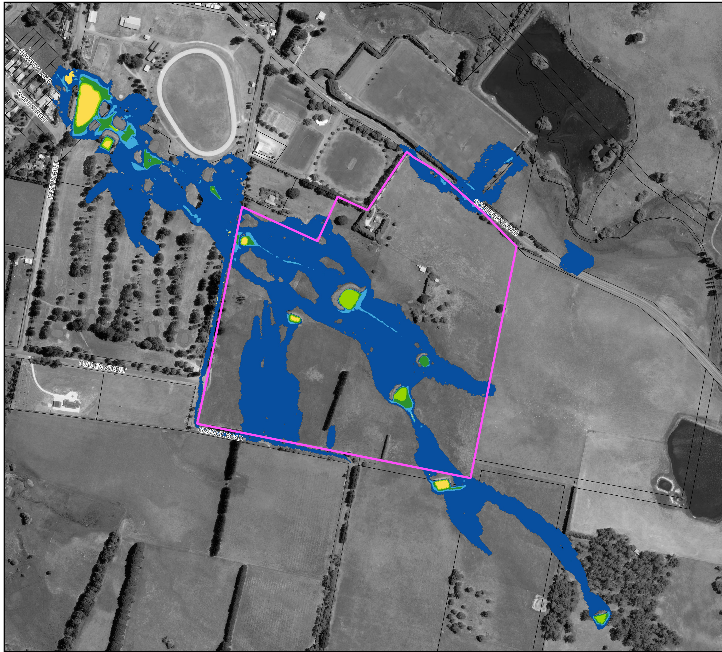
Figure 33 : Flood Hazard for the 0.5% AEP Flood for Existing Conditions
