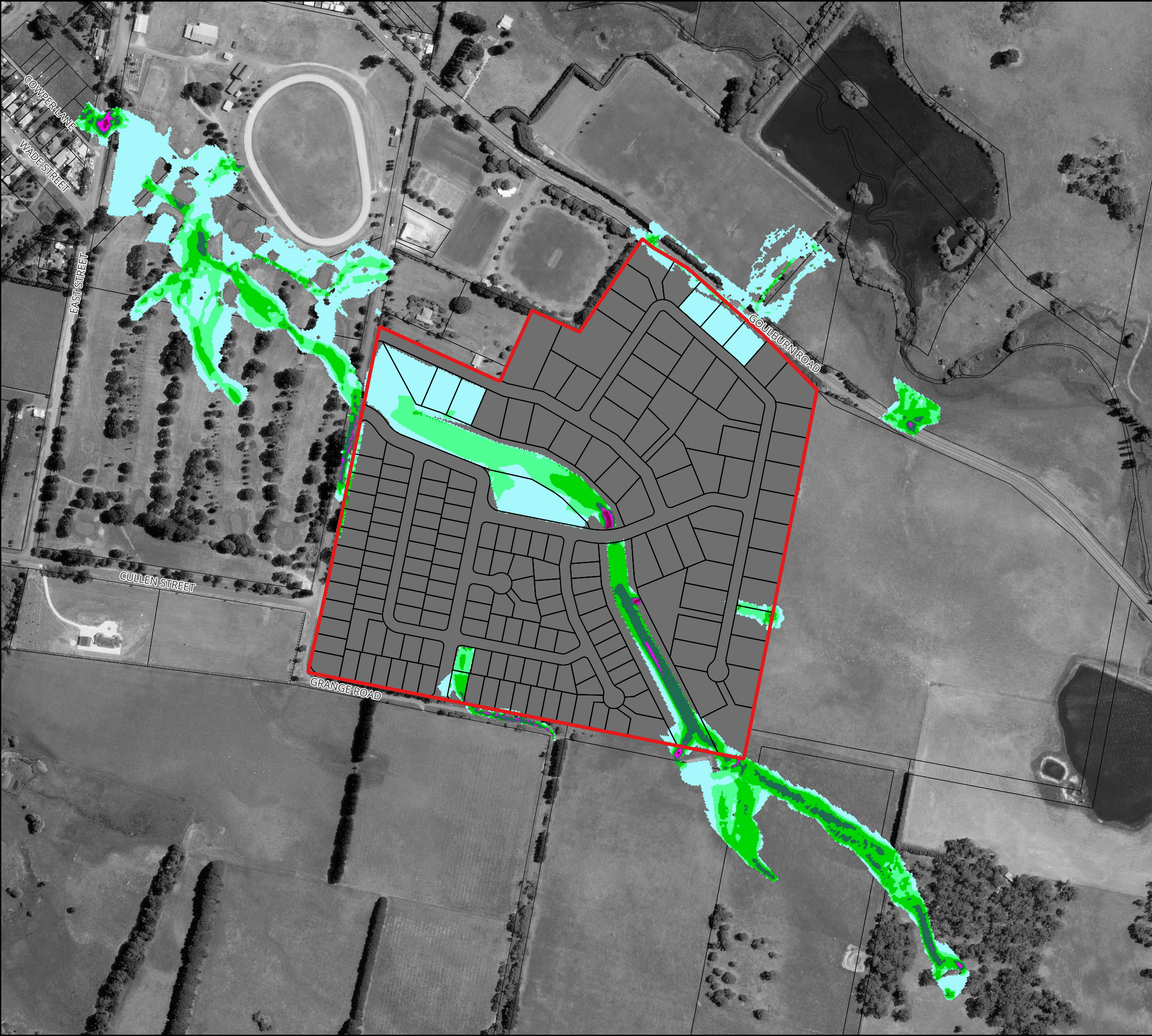
Figure 55 : Peak Flood Velocity for the 0.2% AEP Flood for Proposed Conditions
