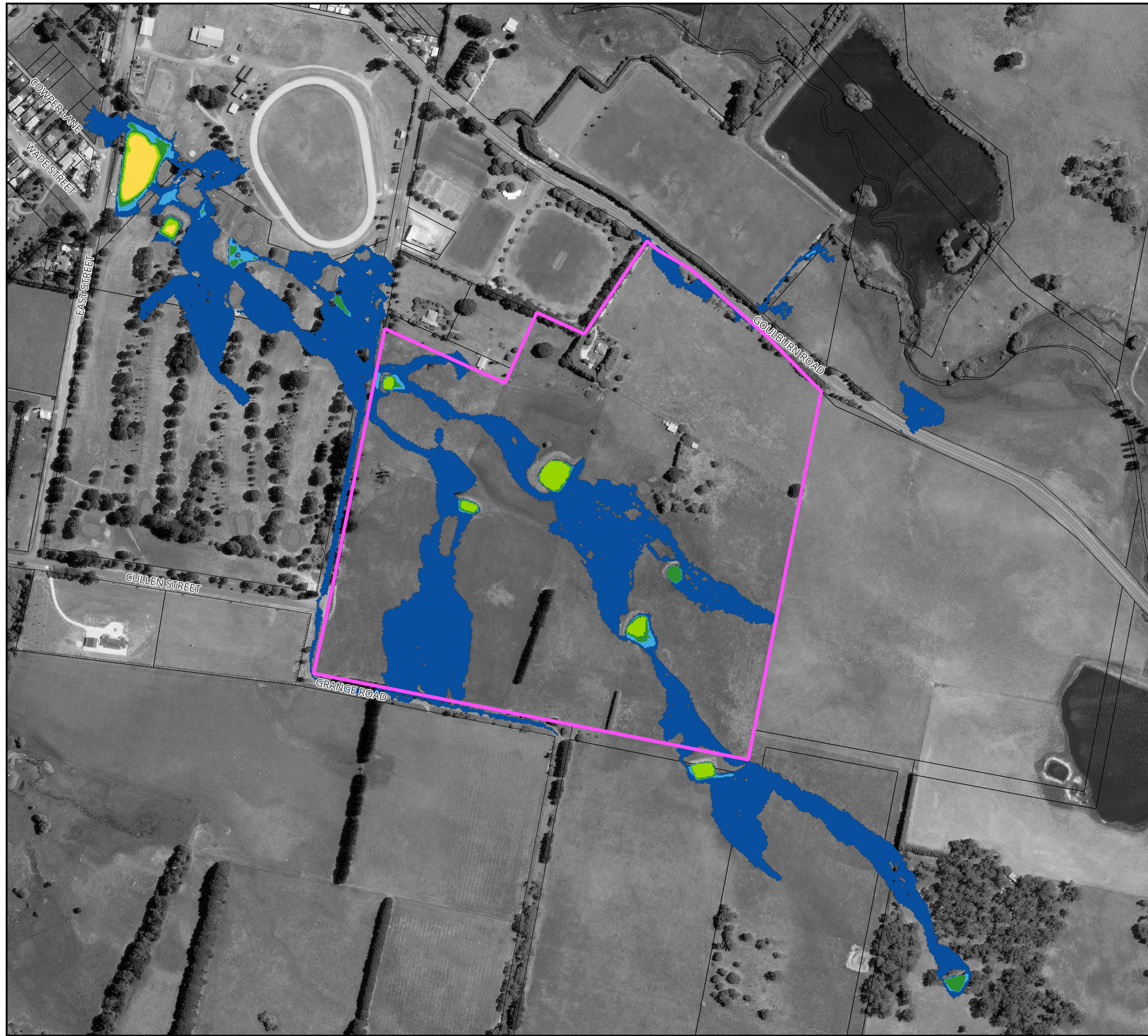
Figure 26 : Flood Hazard for the 63.2% AEP Flood for Existing Conditions
