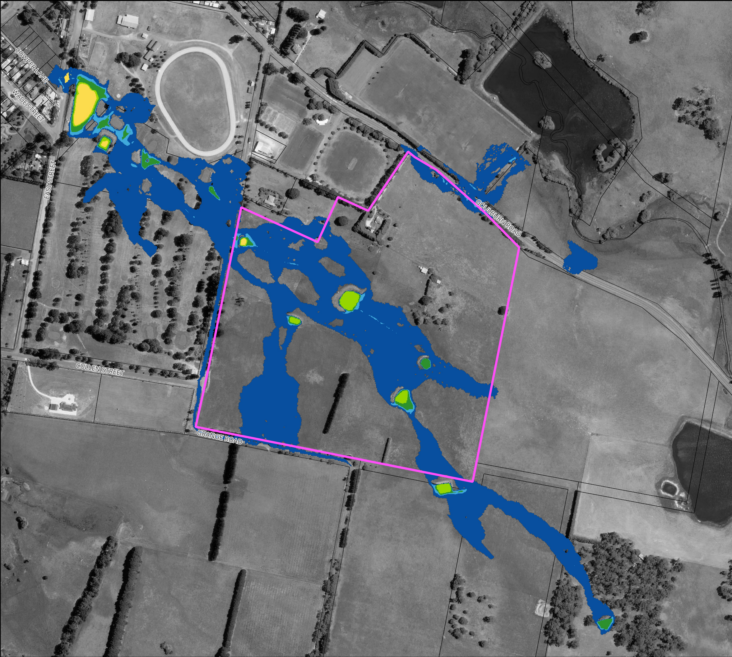
Figure 30 : Flood Hazard for the 5% AEP Flood for Existing Conditions
