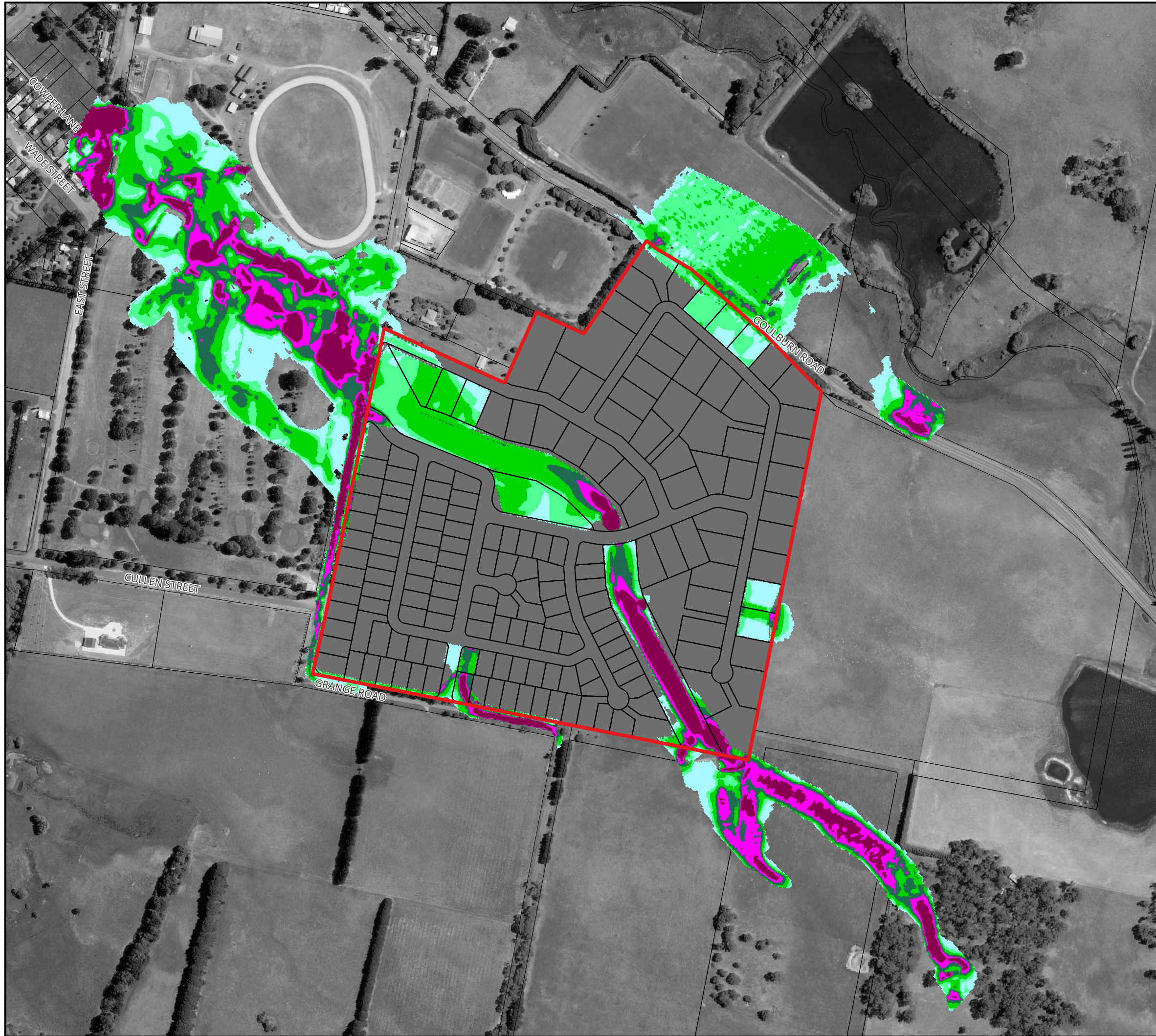
Figure 56 : Peak Flood Velocity for the PMF for Proposed Conditions
