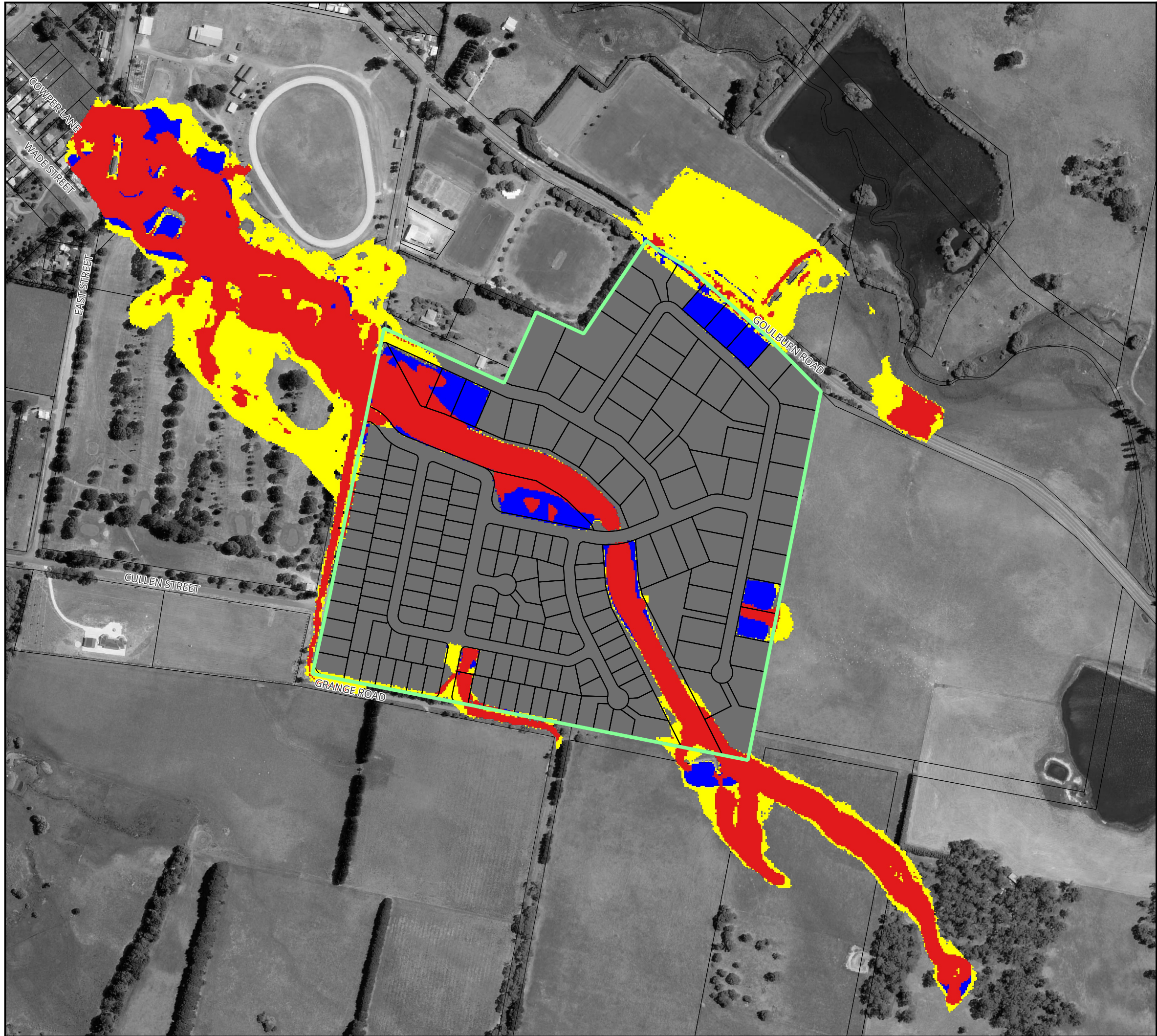
Figure 58 : Hydraulic Categories for the PMF for Proposed Conditions
