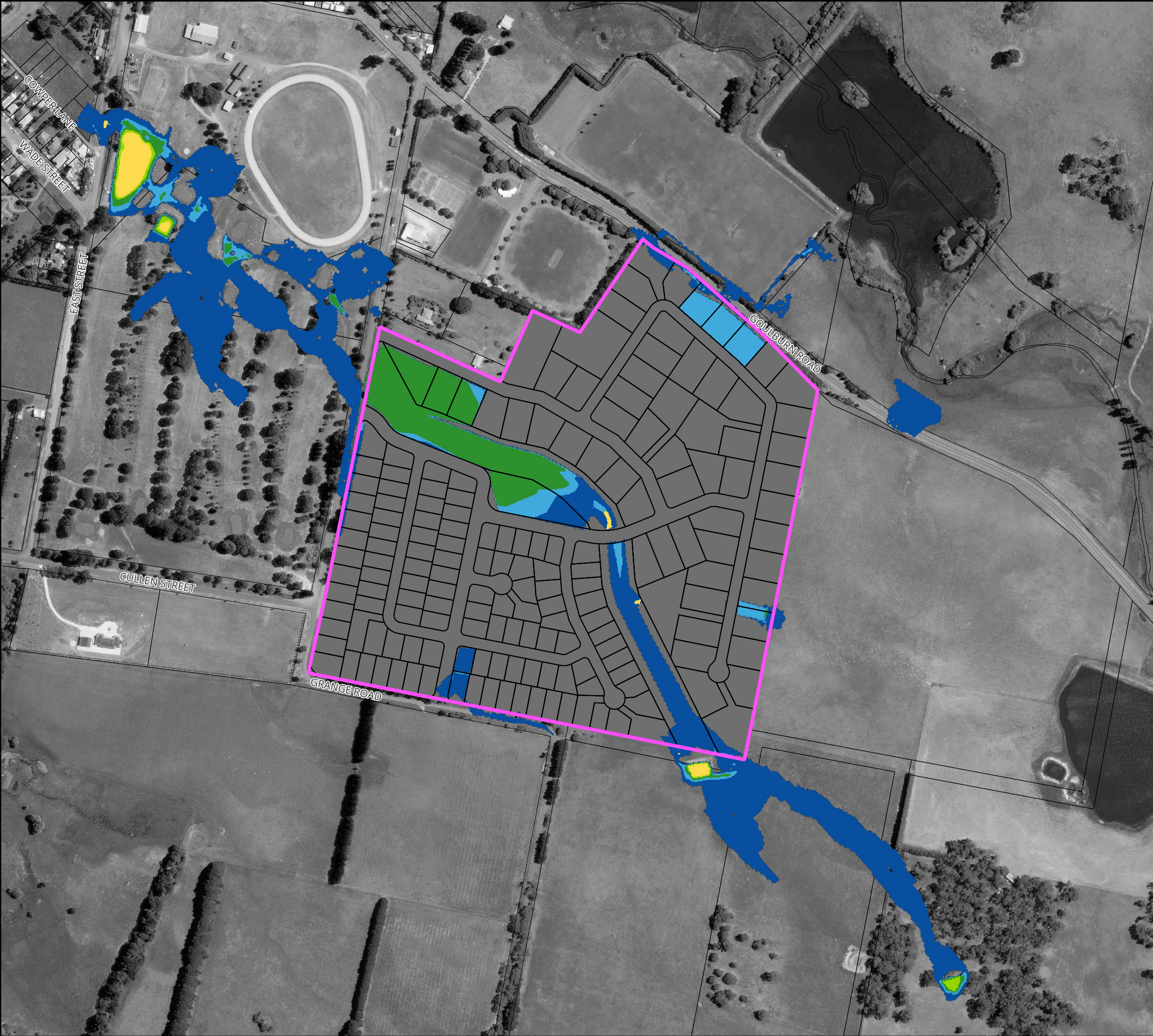
Figure 66 : Flood Hazard for the 0.5% AEP Flood for Proposed Conditions
