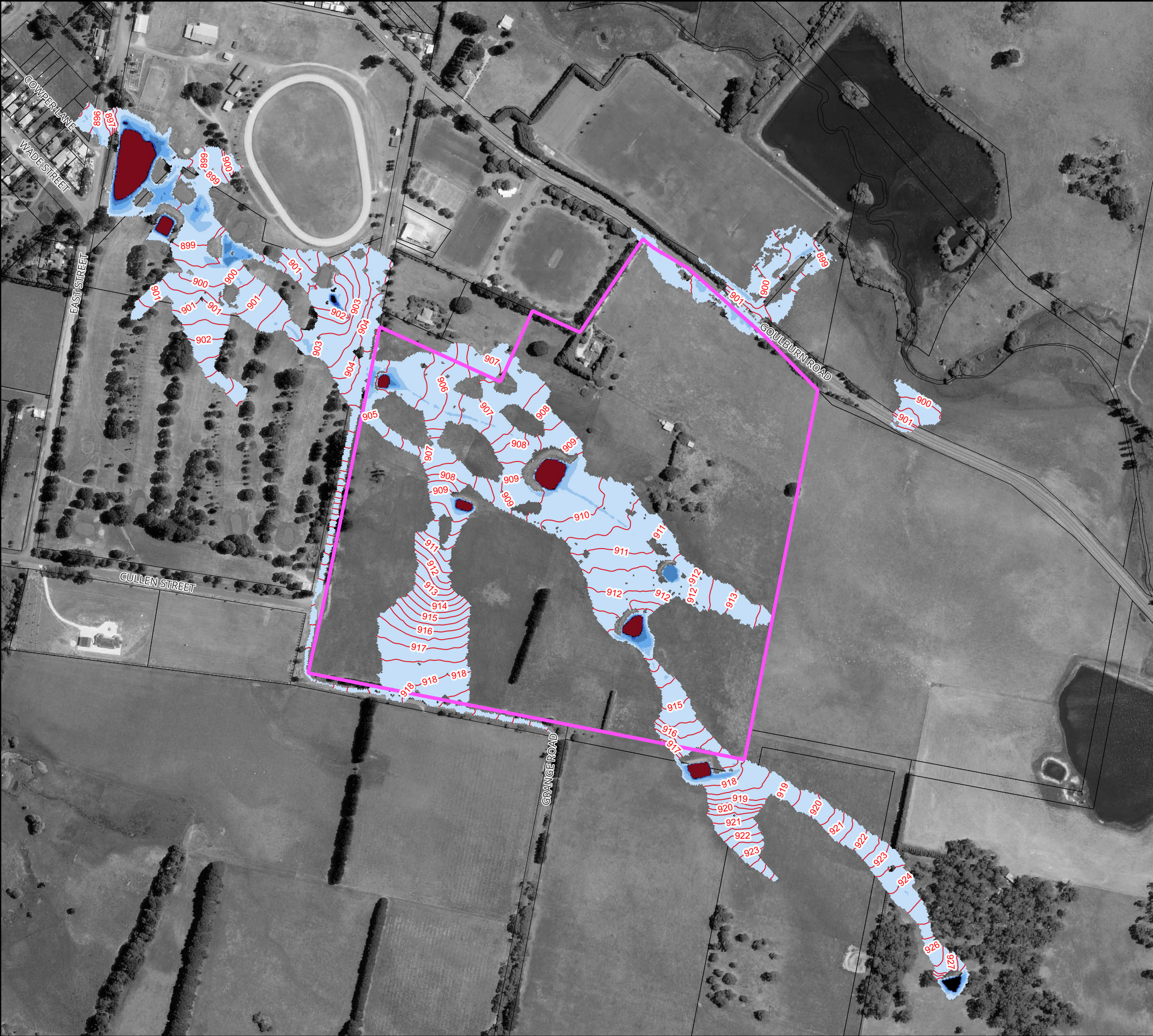
Figure 7 : Peak Floodwater Depths and Levels for the 10% AEP Flood for Existing Conditions
