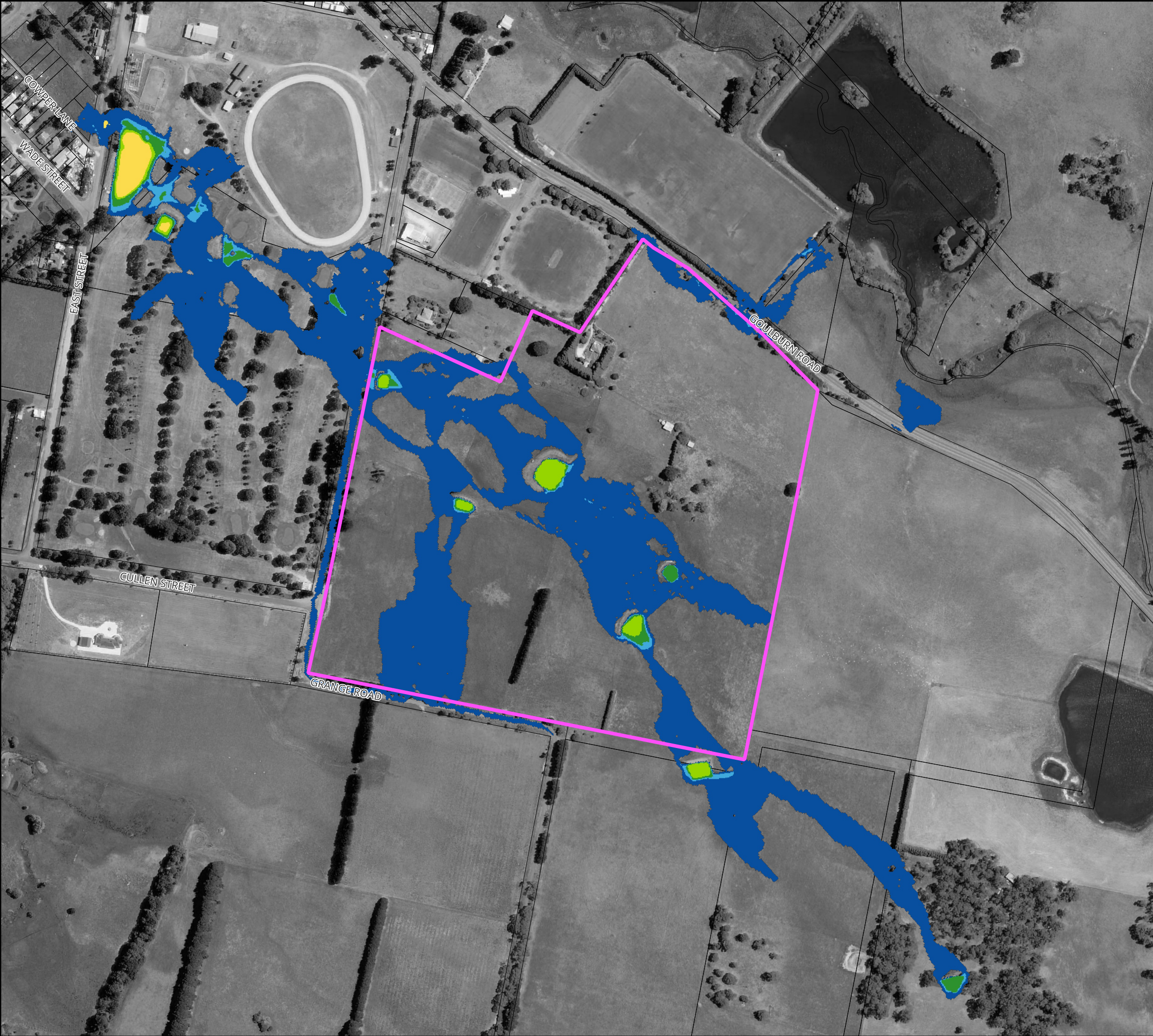
Figure 28 : Flood Hazard for the 20% AEP Flood for Existing Conditions
