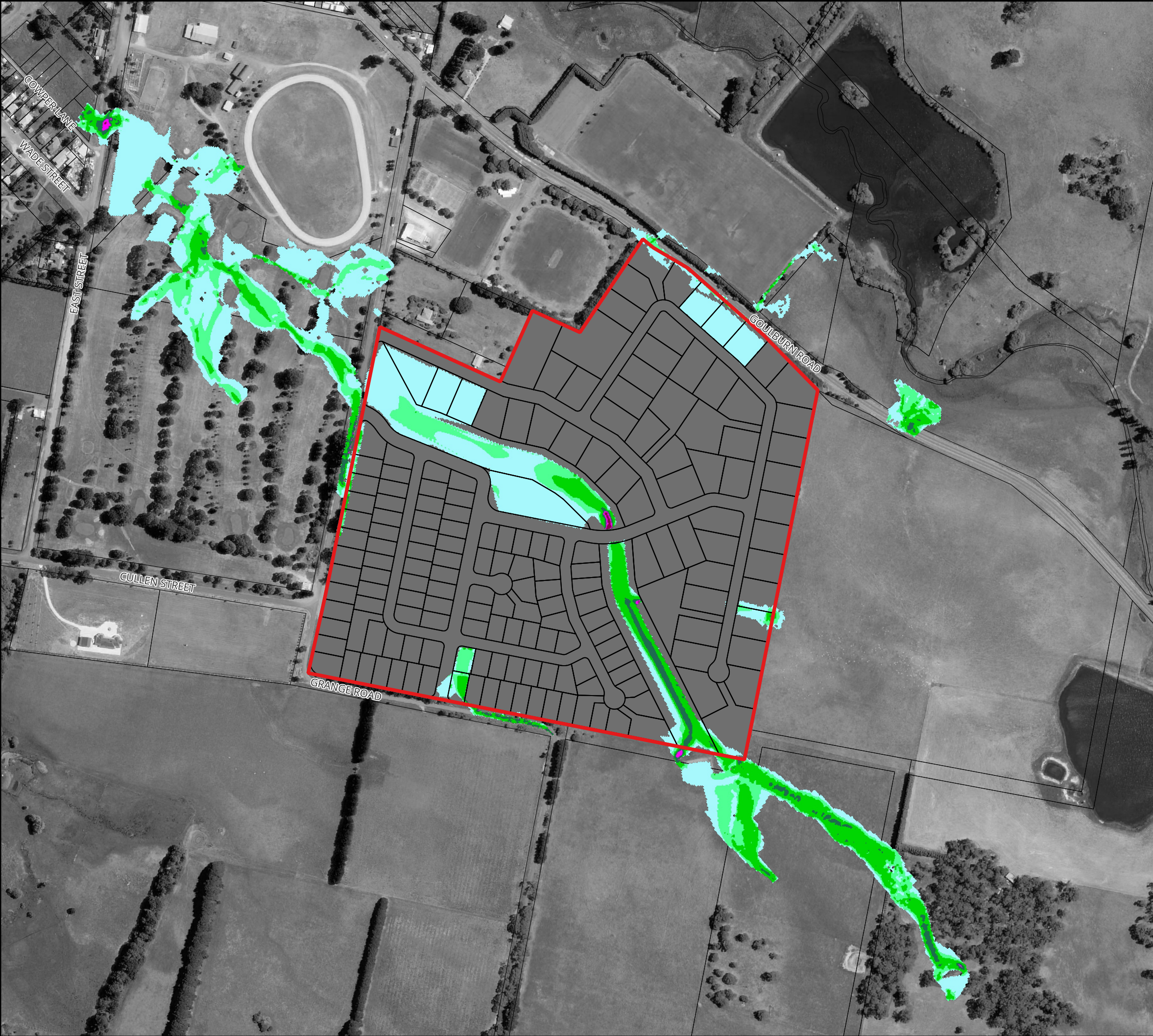
Figure 52 : Peak Flood Velocity for the 2% AEP Flood for Proposed Conditions
