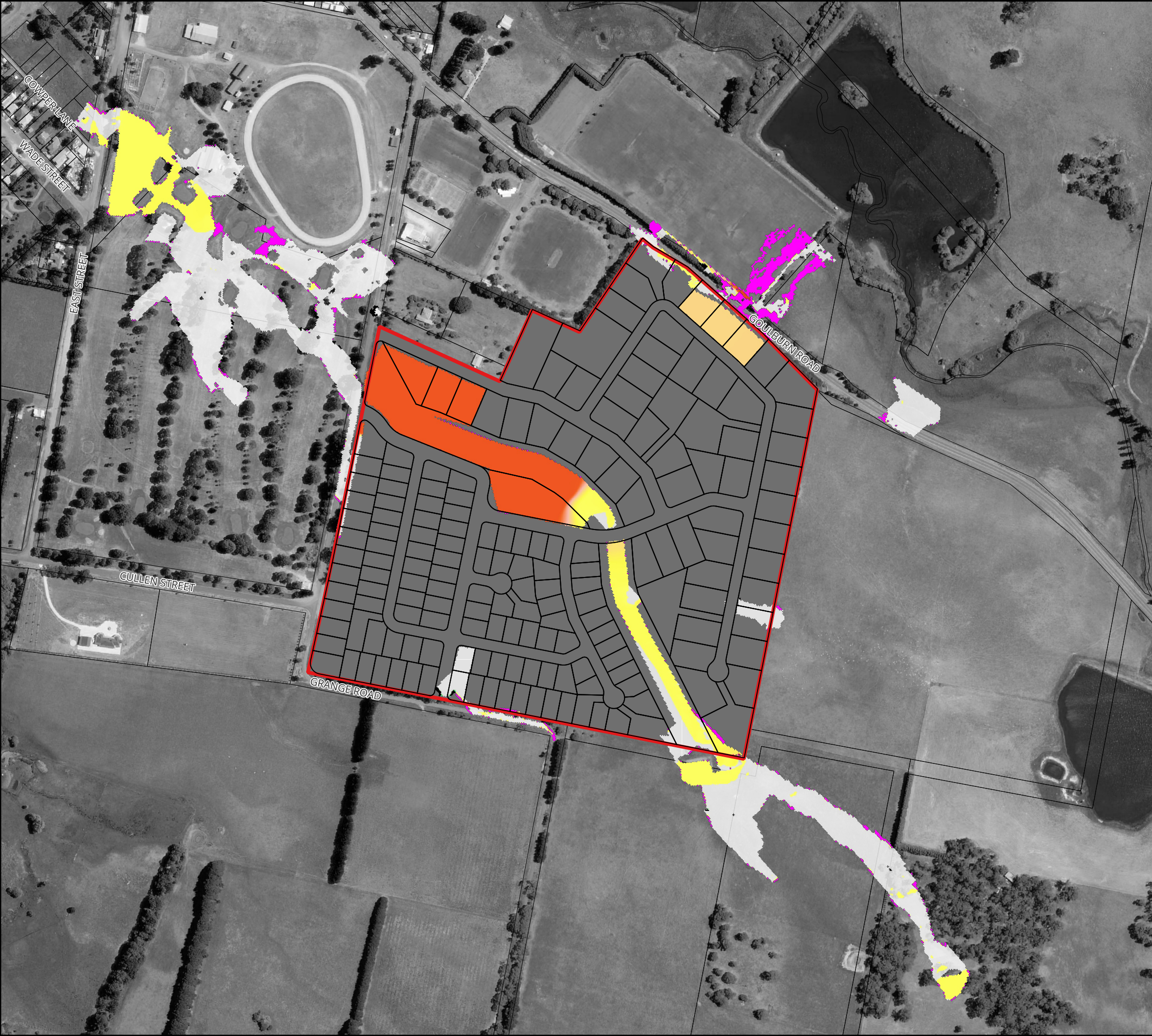
Figure 91 : Predicted Change in Peak 1% AEP Flood Levels as a result of Climate Change using the 0.2% AEP Event as a Proxy
