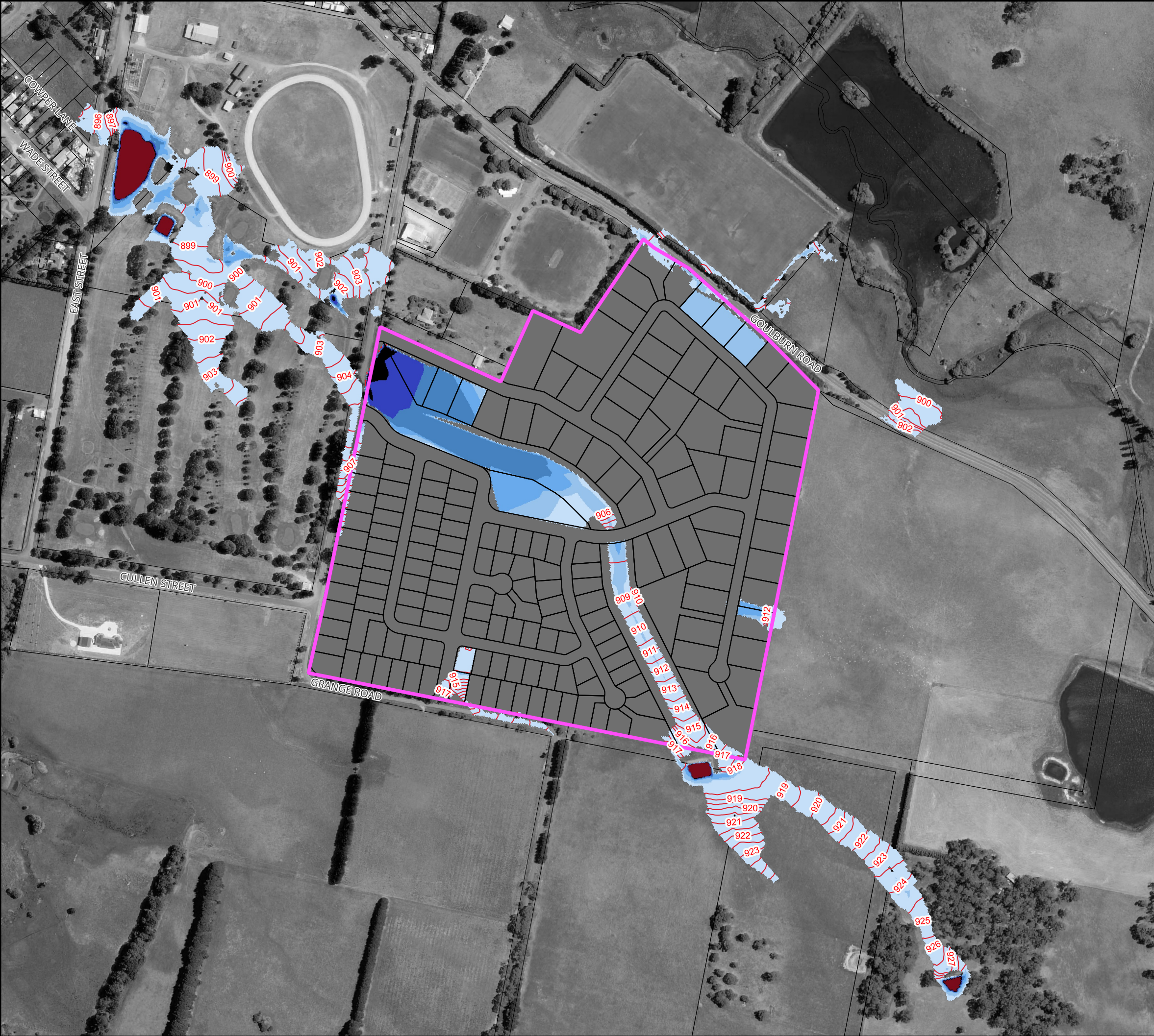
Figure 93 : Peak Floodwater Depths and Levels for the 1% AEP Flood for Proposed Conditions with High Culvert Blockage
