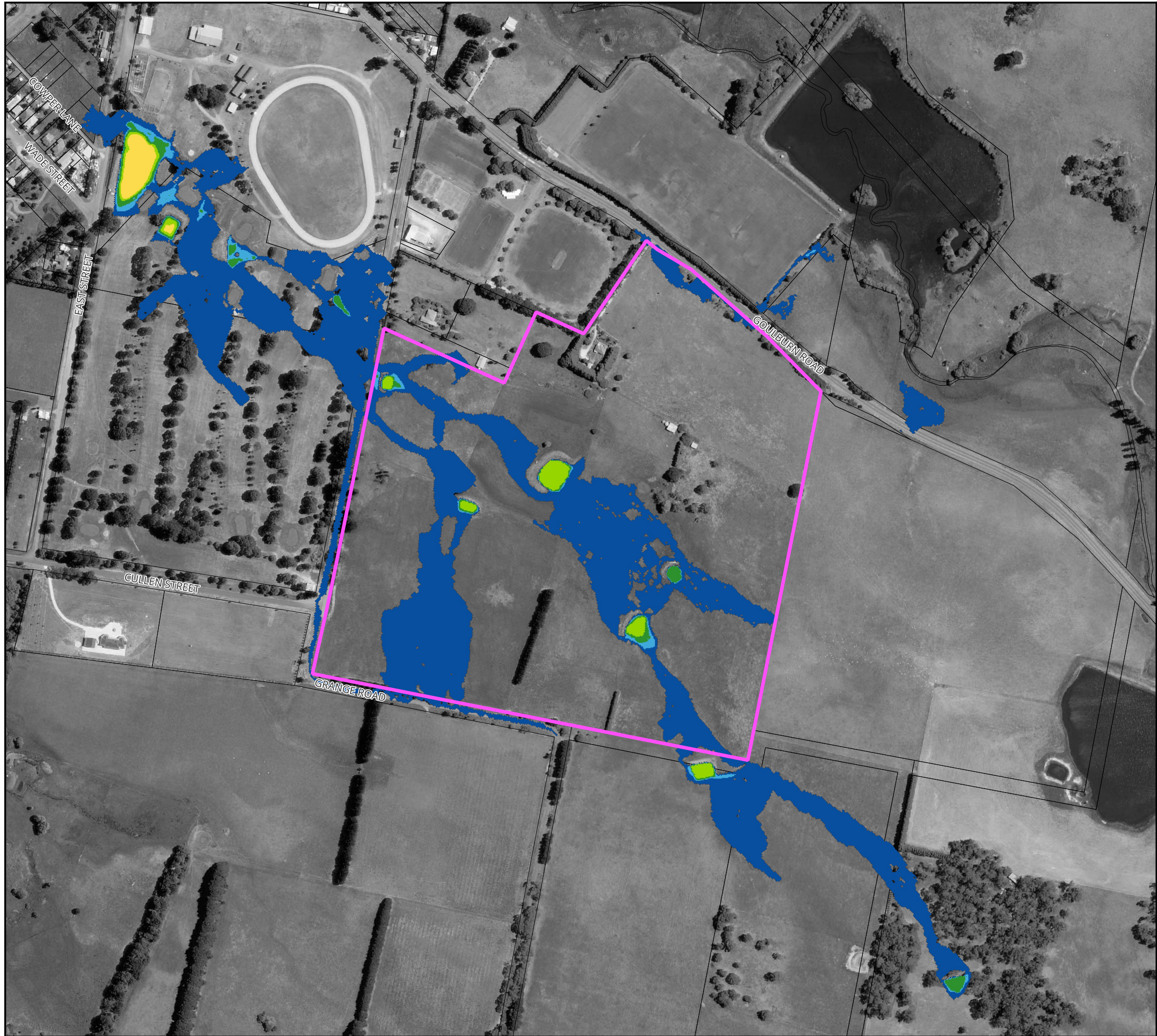
Figure 27 : Flood Hazard for the 50% AEP Flood for Existing Conditions
