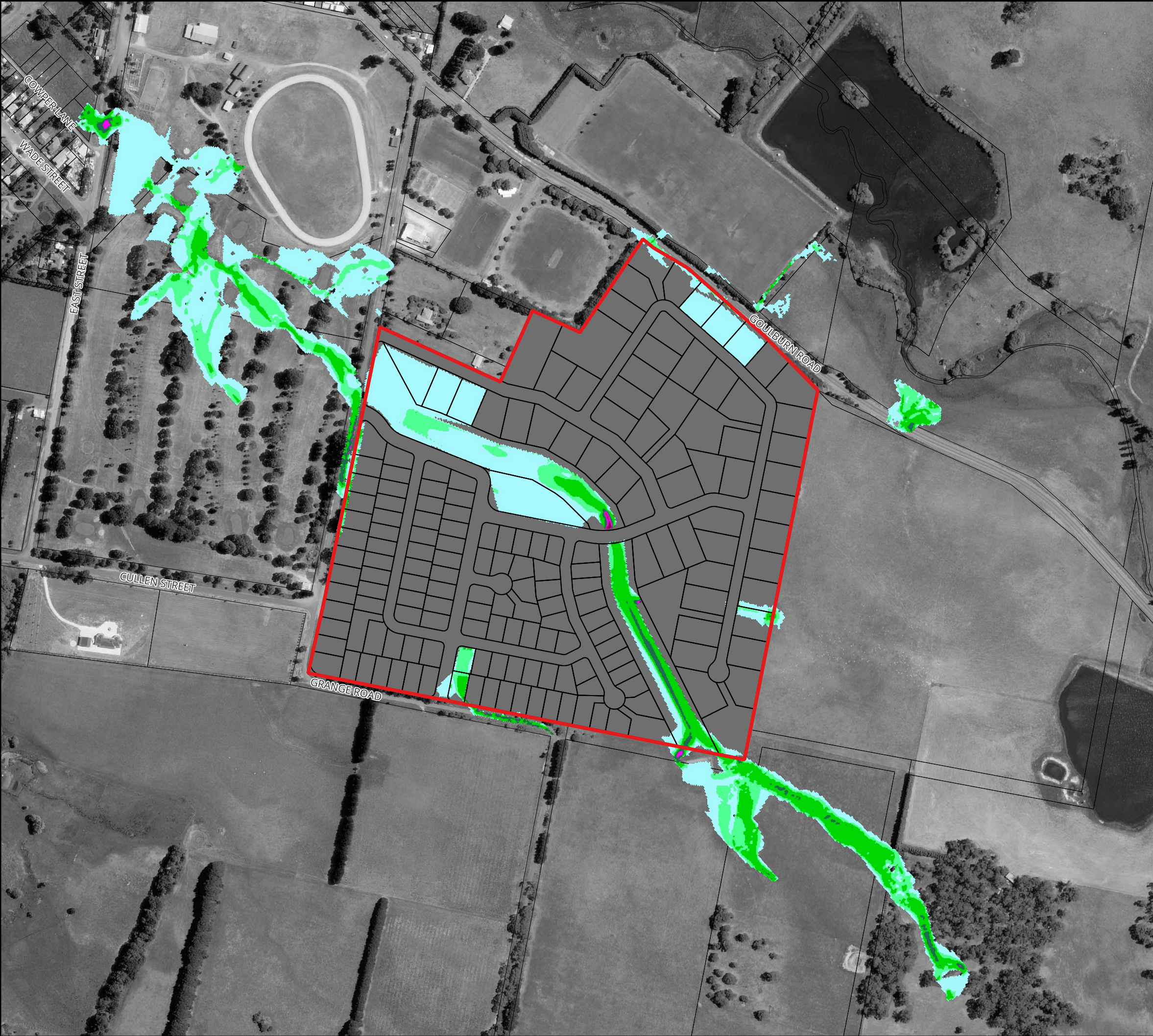
Figure 51 : Peak Flood Velocity for the 5% AEP Flood for Proposed Conditions
