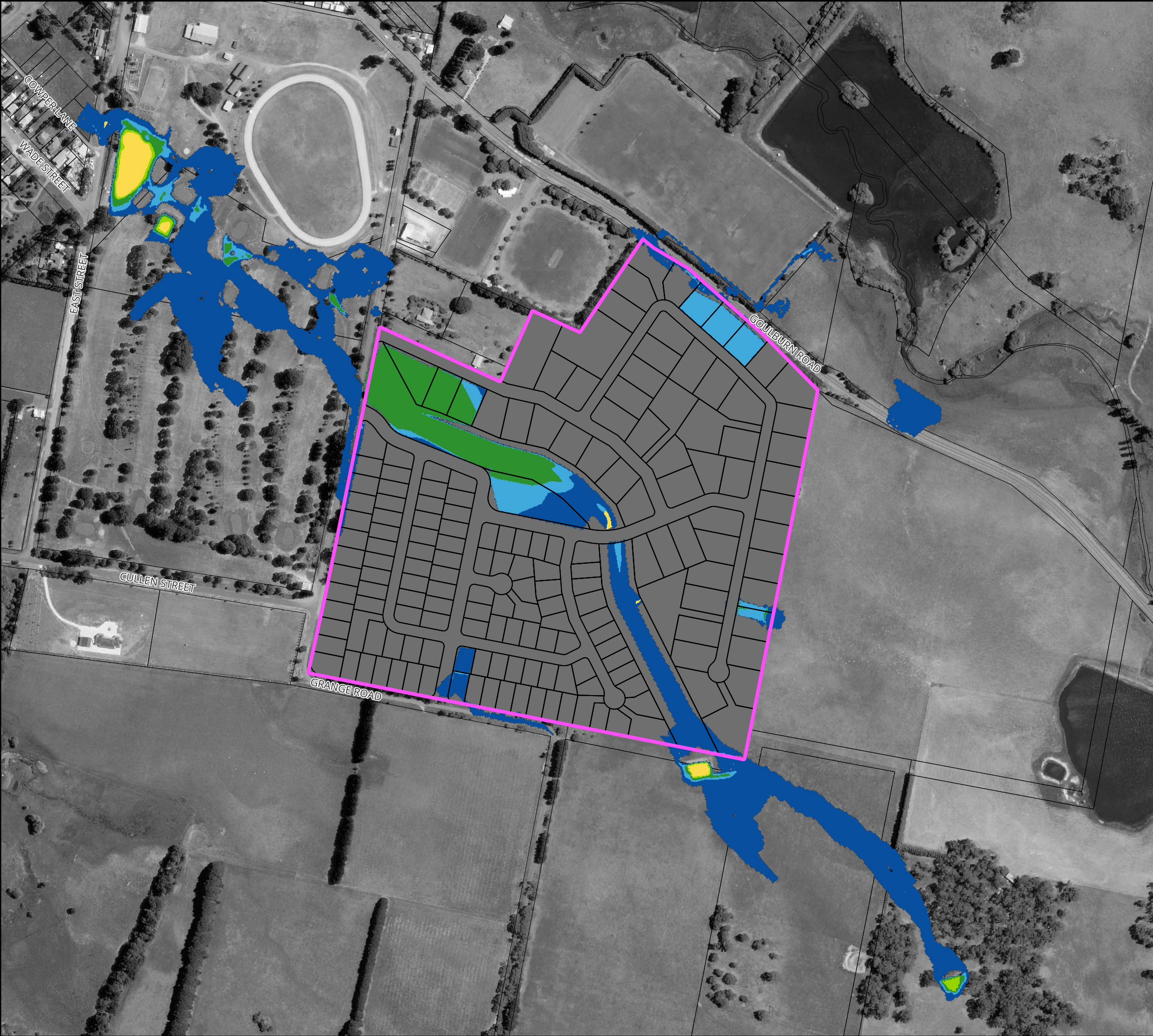
Figure 65 : Flood Hazard for the 1% AEP Flood for Proposed Conditions
