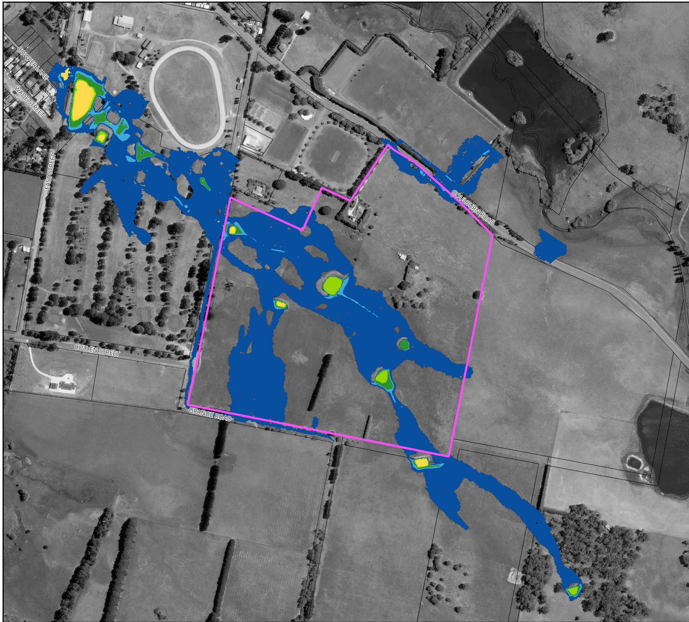
Figure 32 : Flood Hazard for the 1% AEP Flood for Existing Conditions
