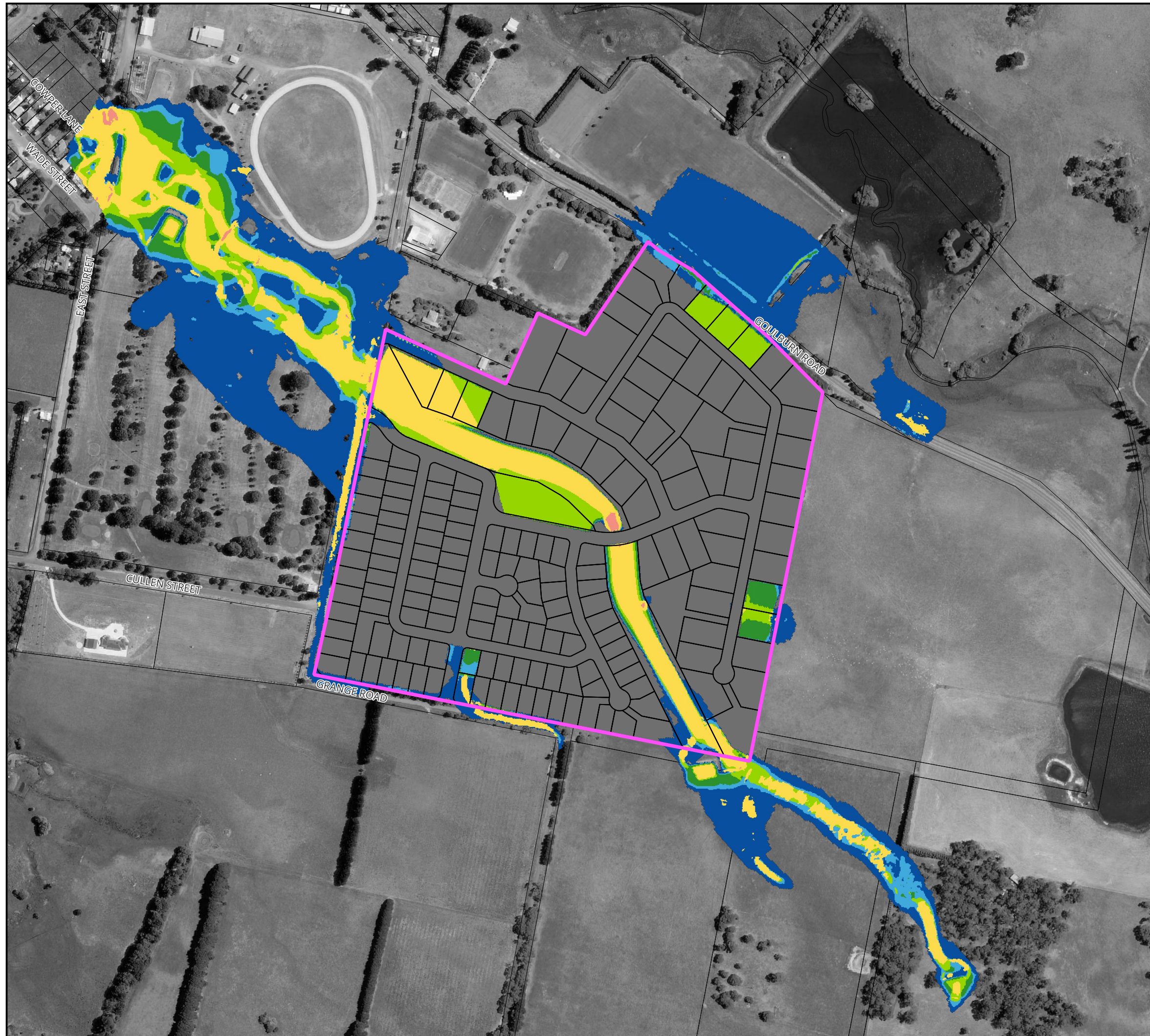
Figure 68 : Flood Hazard for the PMF for Proposed Conditions
