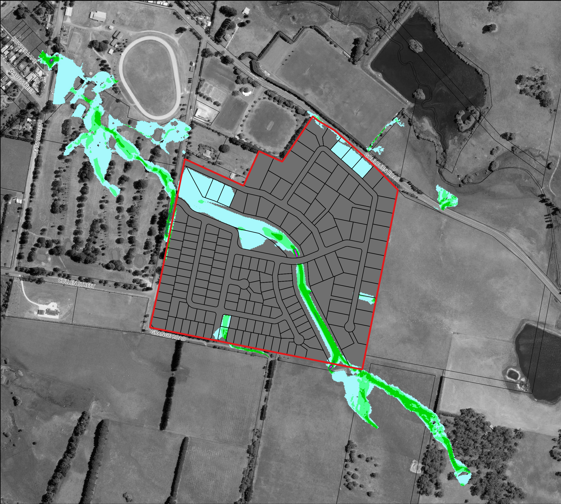
Figure 49 : Peak Flood Velocity for the 20% AEP Flood for Proposed Conditions
