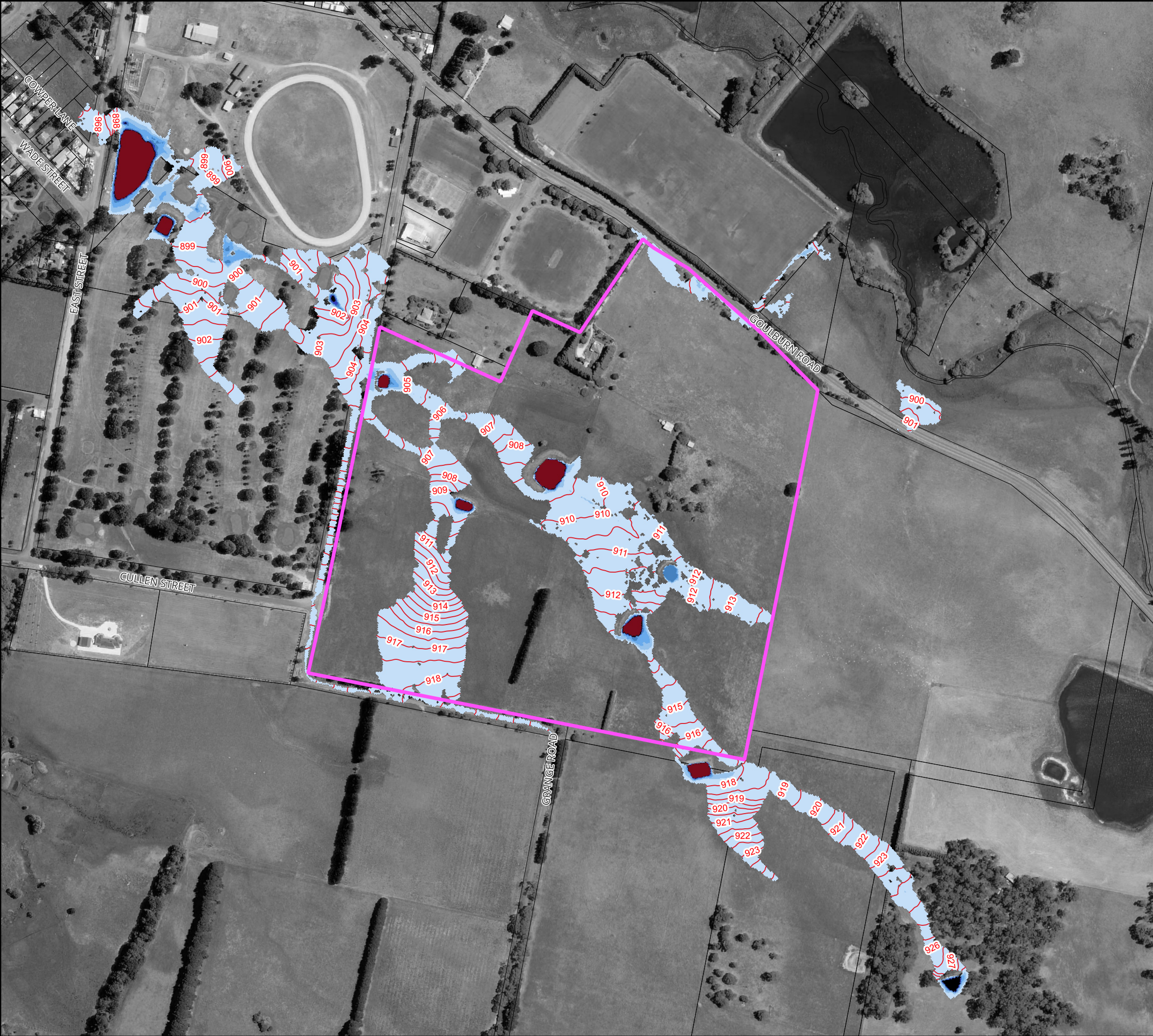
Figure 5 : Peak Floodwater Depths and Levels for the 50% AEP Flood for Existing Conditions
