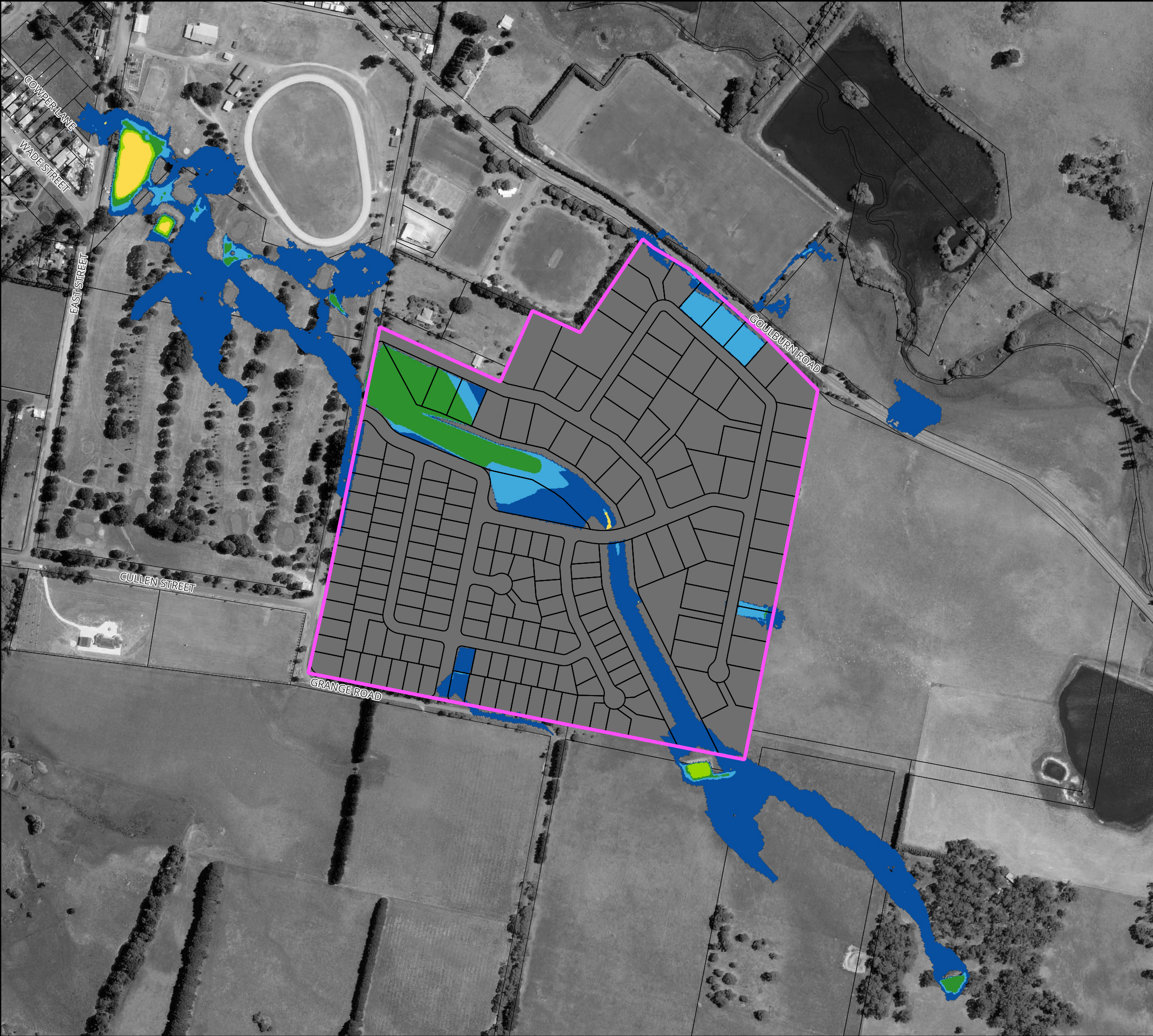
Figure 64 : Flood Hazard for the 2% AEP Flood for Proposed Conditions
