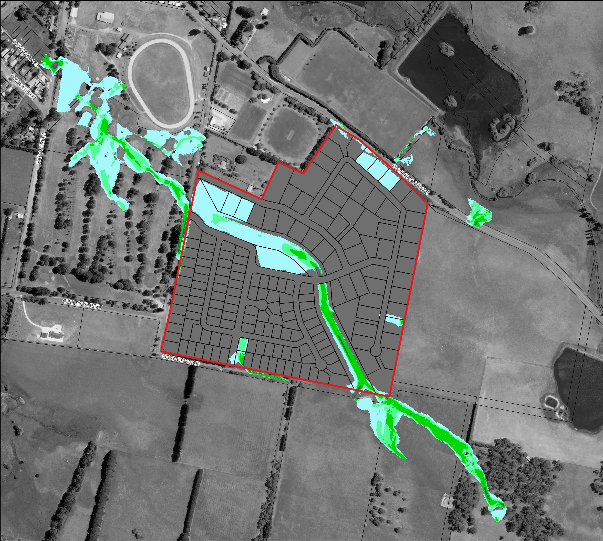
Figure 50 : Peak Flood Velocity for the 10% AEP Flood for Proposed Conditions
