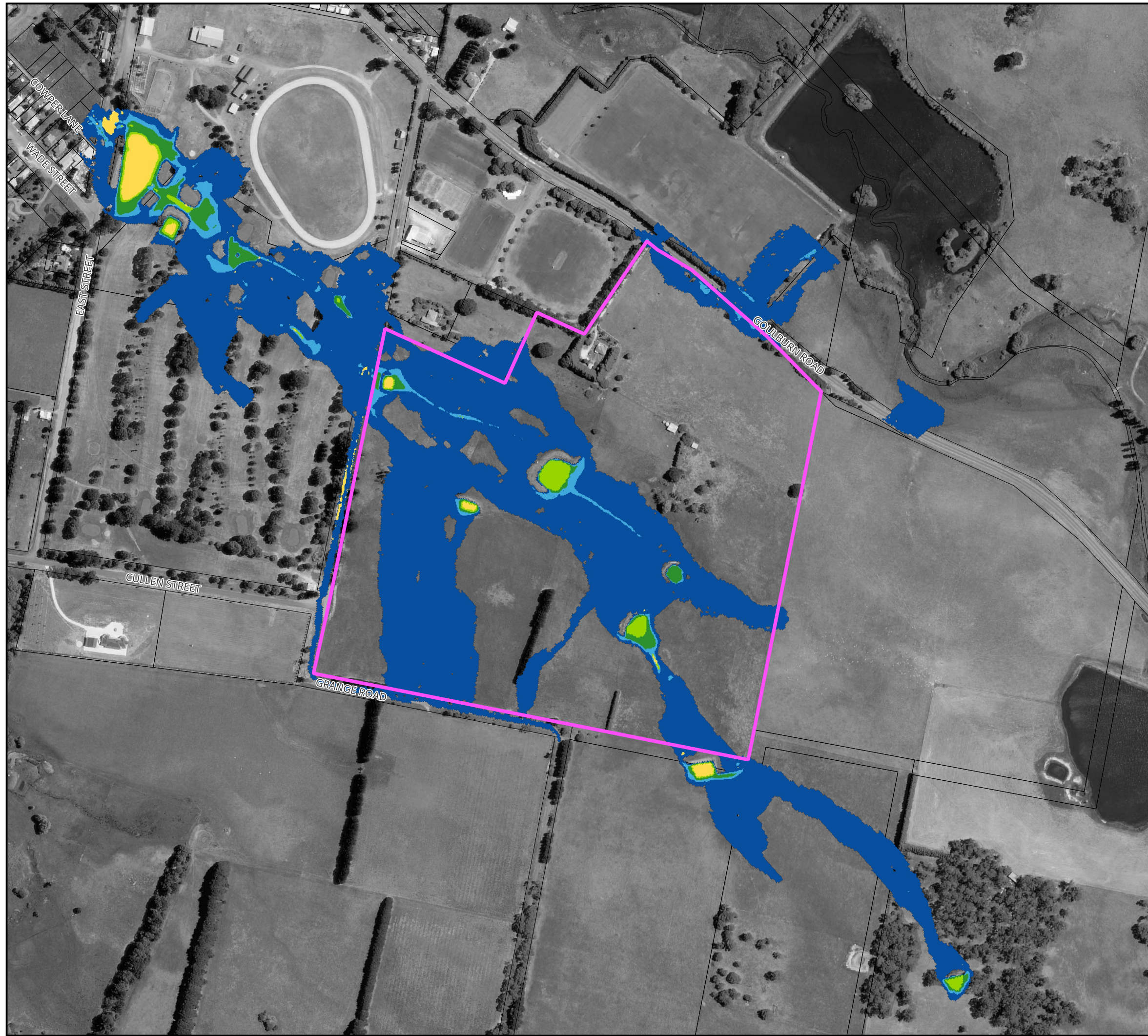
Figure 34 : Flood Hazard for the 0.2% AEP Flood for Existing Conditions
