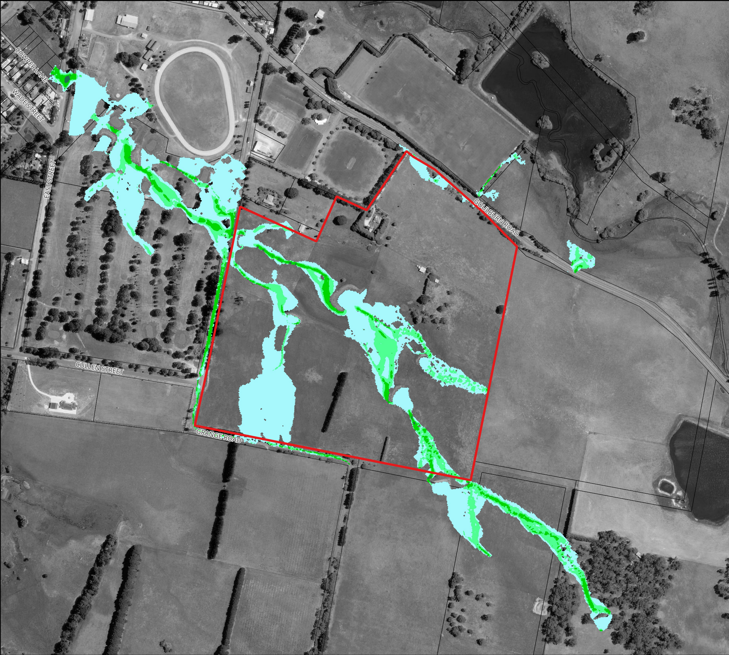
Figure 14 : Peak Flood Velocity for the 63.2% AEP Flood for Existing Conditions
