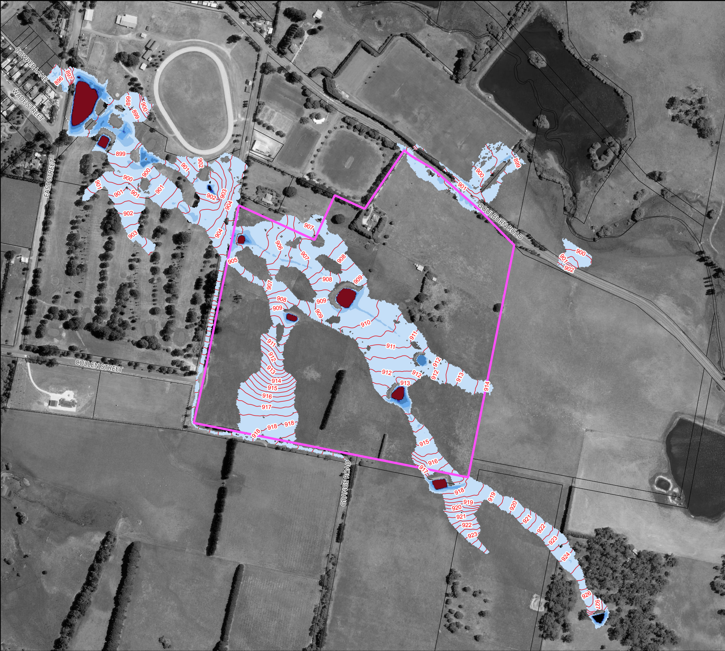
Figure 8 : Peak Floodwater Depths and Levels for the 5% AEP Flood for Existing Conditions
