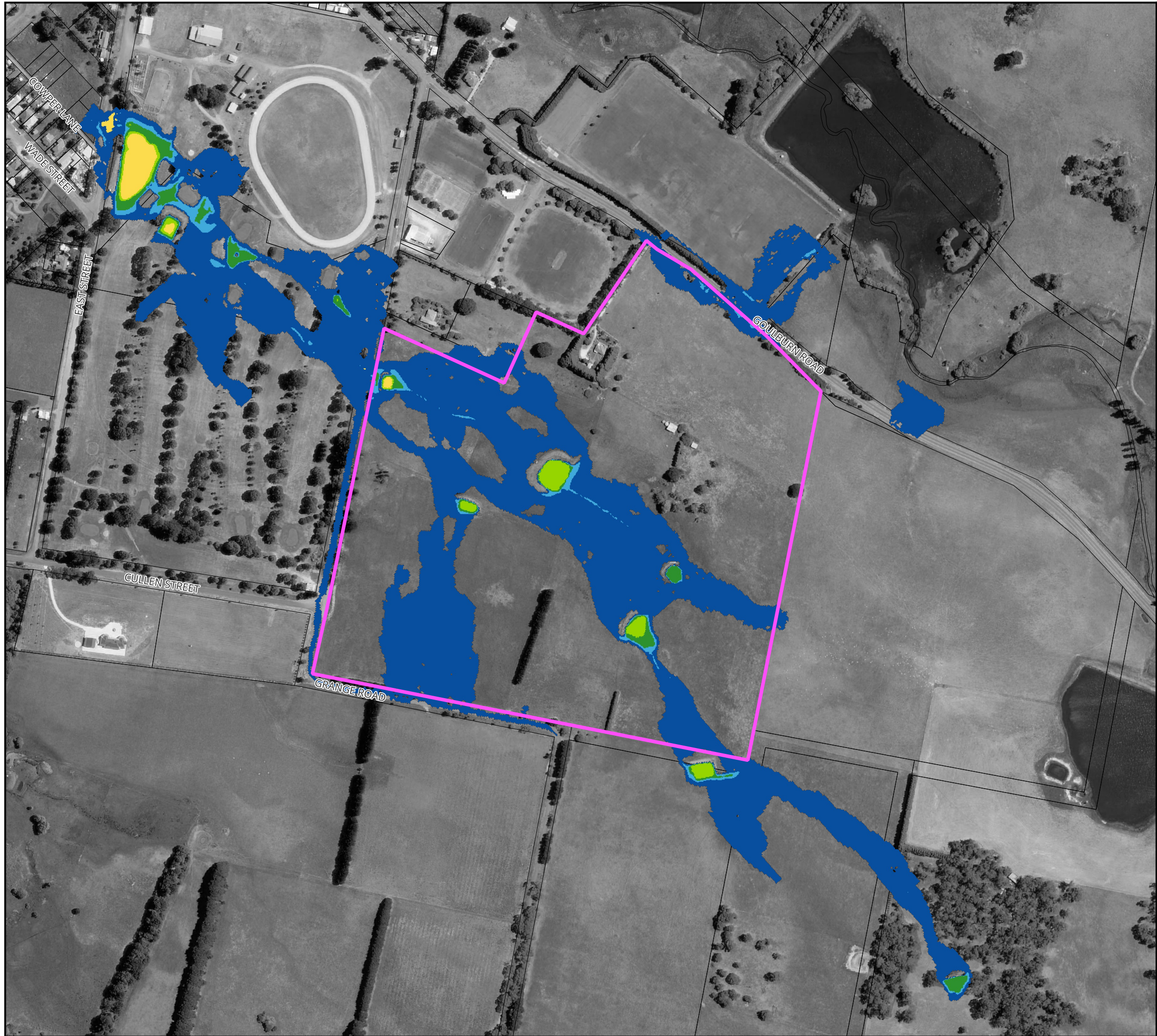
Figure 31 : Flood Hazard for the 2% AEP Flood for Existing Conditions
