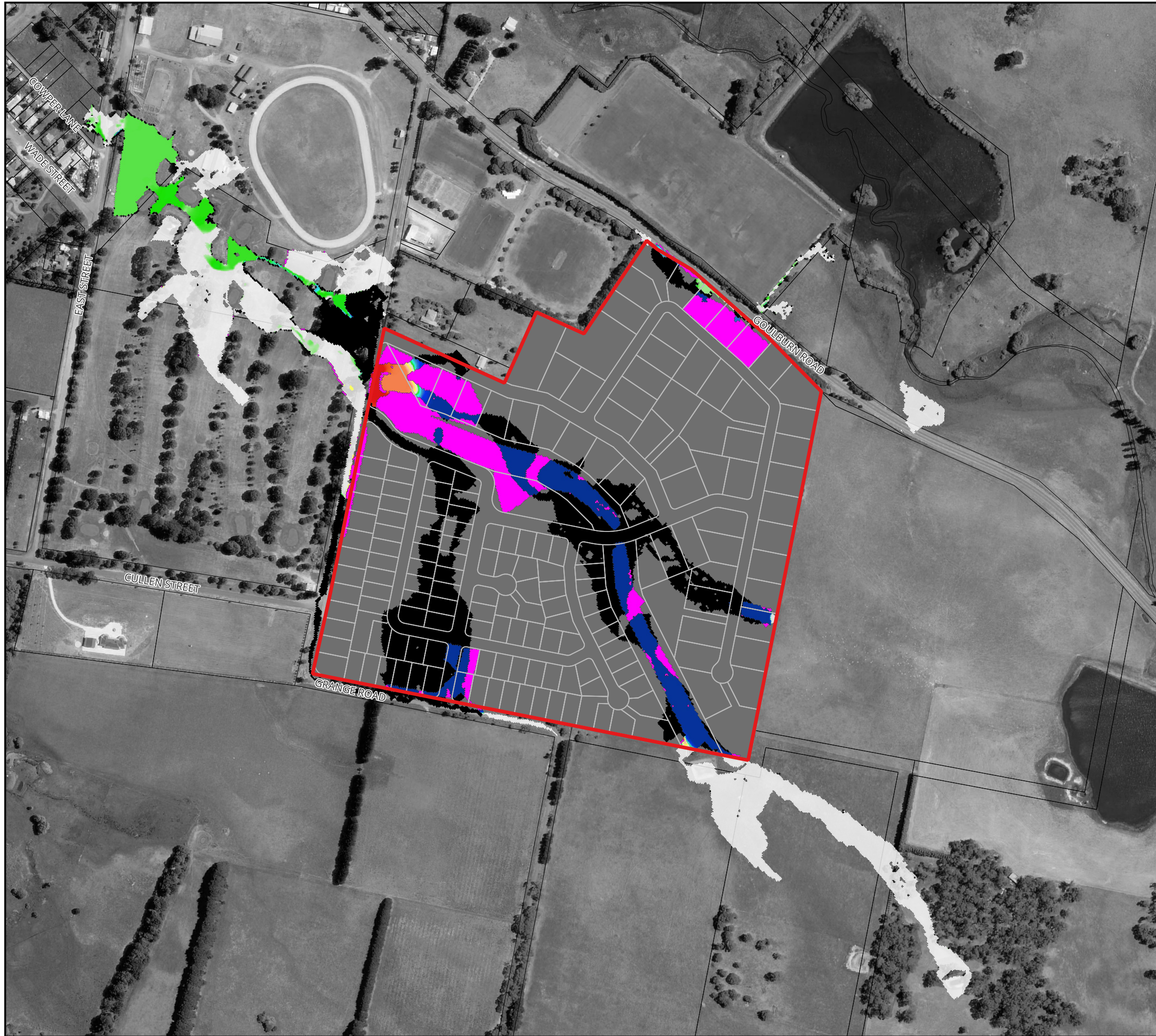
Figure 69 : Predicted Change in Peak 63.2% AEP Flood Levels
