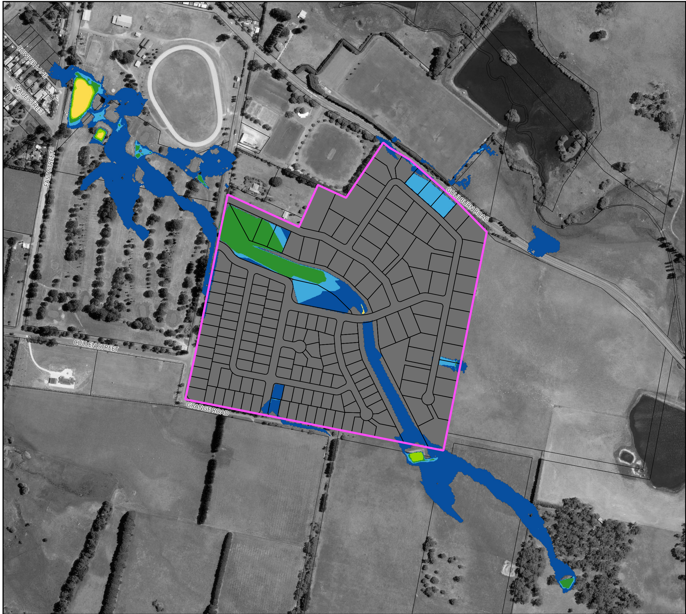
Figure 63 : Flood Hazard for the 5% AEP Flood for Proposed Conditions
