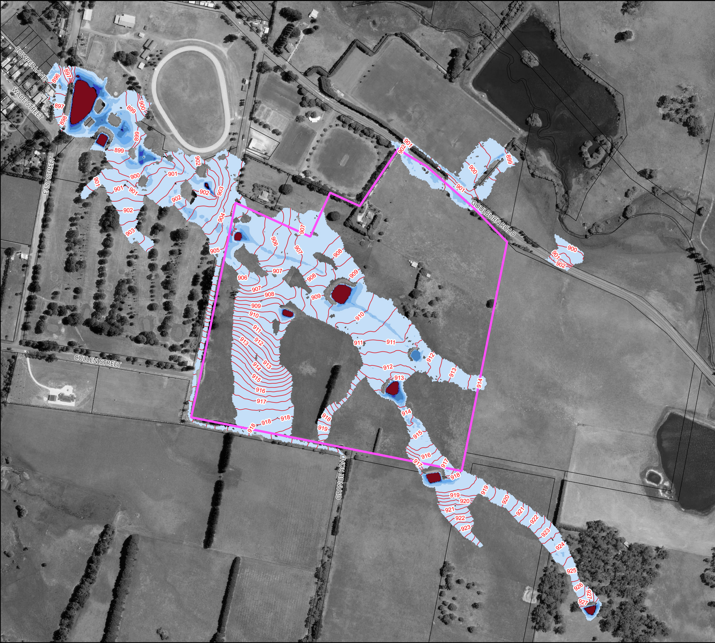
Figure 12 : Peak Floodwater Depths and Levels for the 0.2% AEP Flood for Existing Conditions
