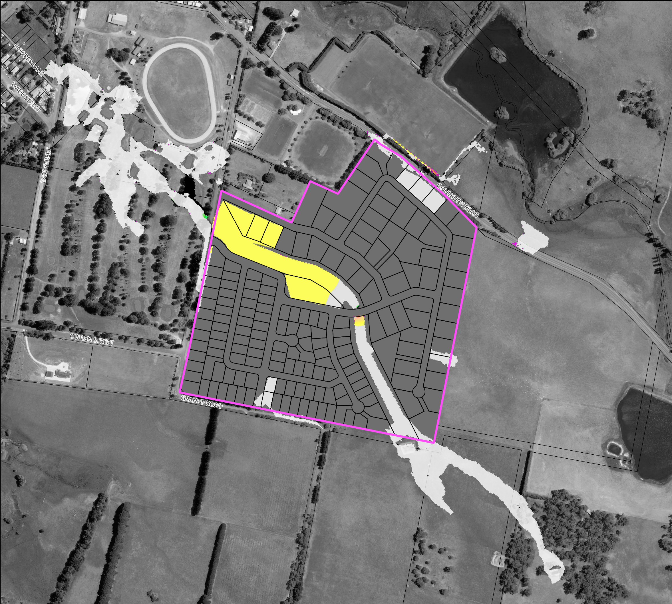
Figure 94 : Predicted Change in Peak 1% AEP Flood Levels as a result High Culvert Blockage
