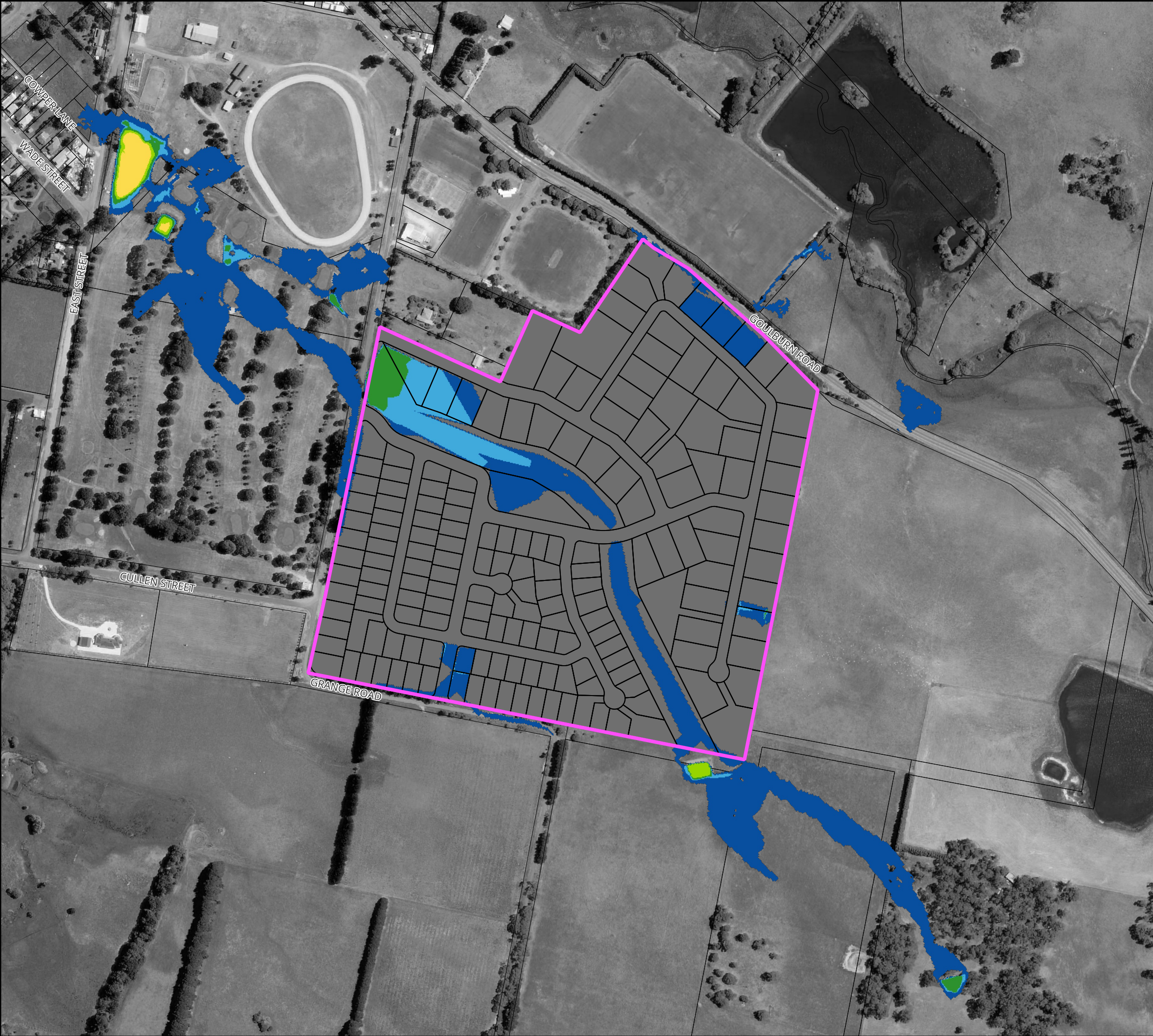
Figure 60 : Flood Hazard for the 50% AEP Flood for Proposed Conditions
