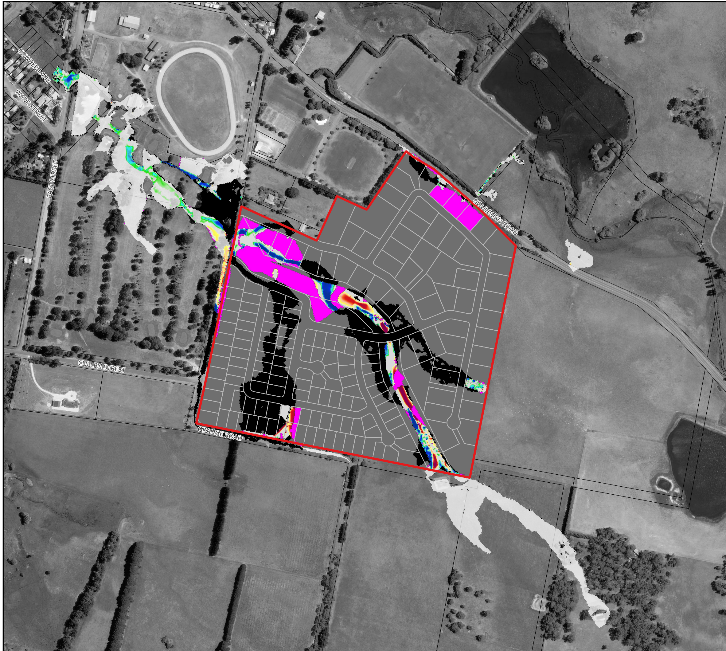
Figure 79 : Predicted Change in Peak 63.2% AEP Flood Velocity
