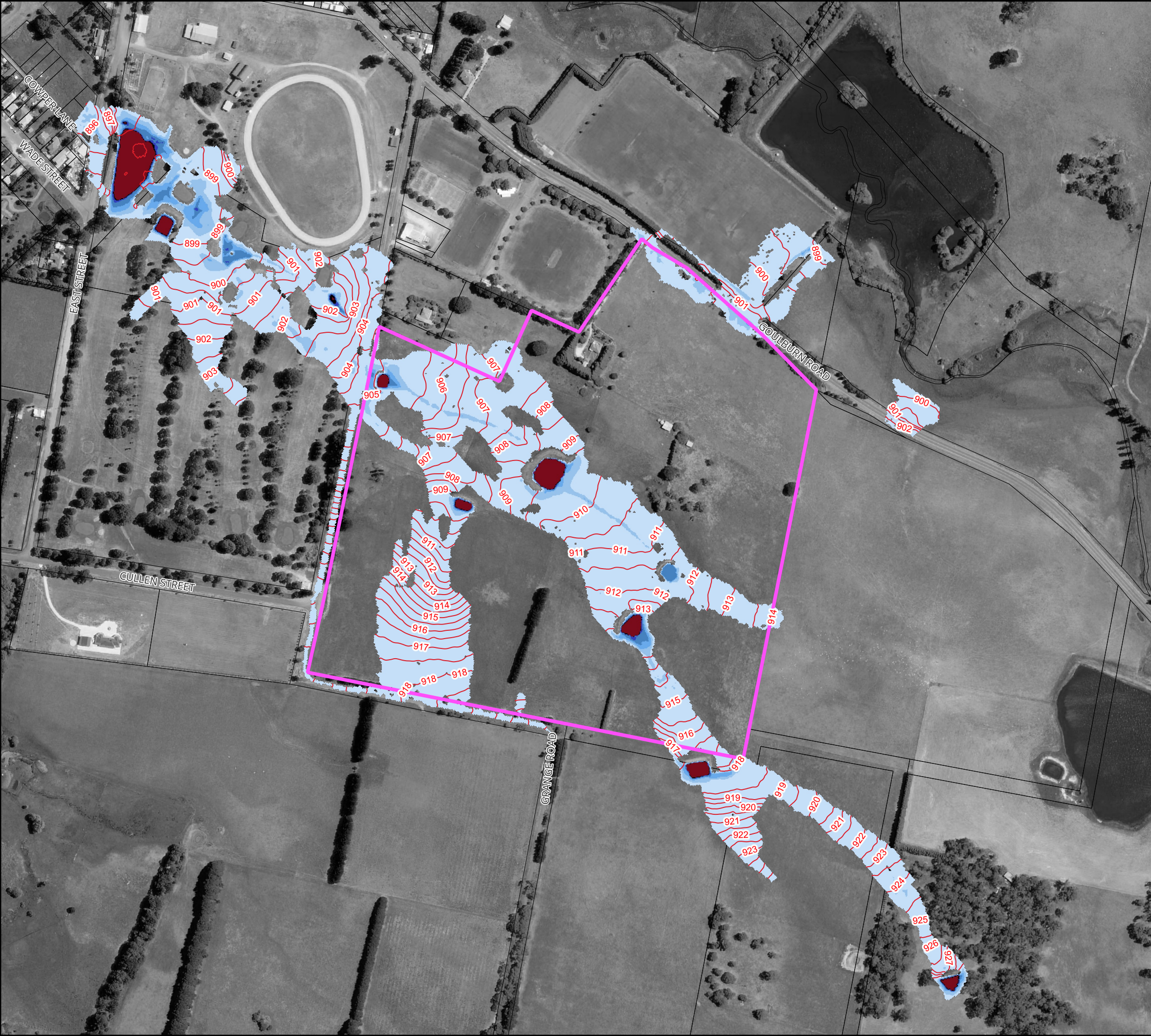
Figure 10 : Peak Floodwater Depths and Levels for the 1% AEP Flood for Existing Conditions
