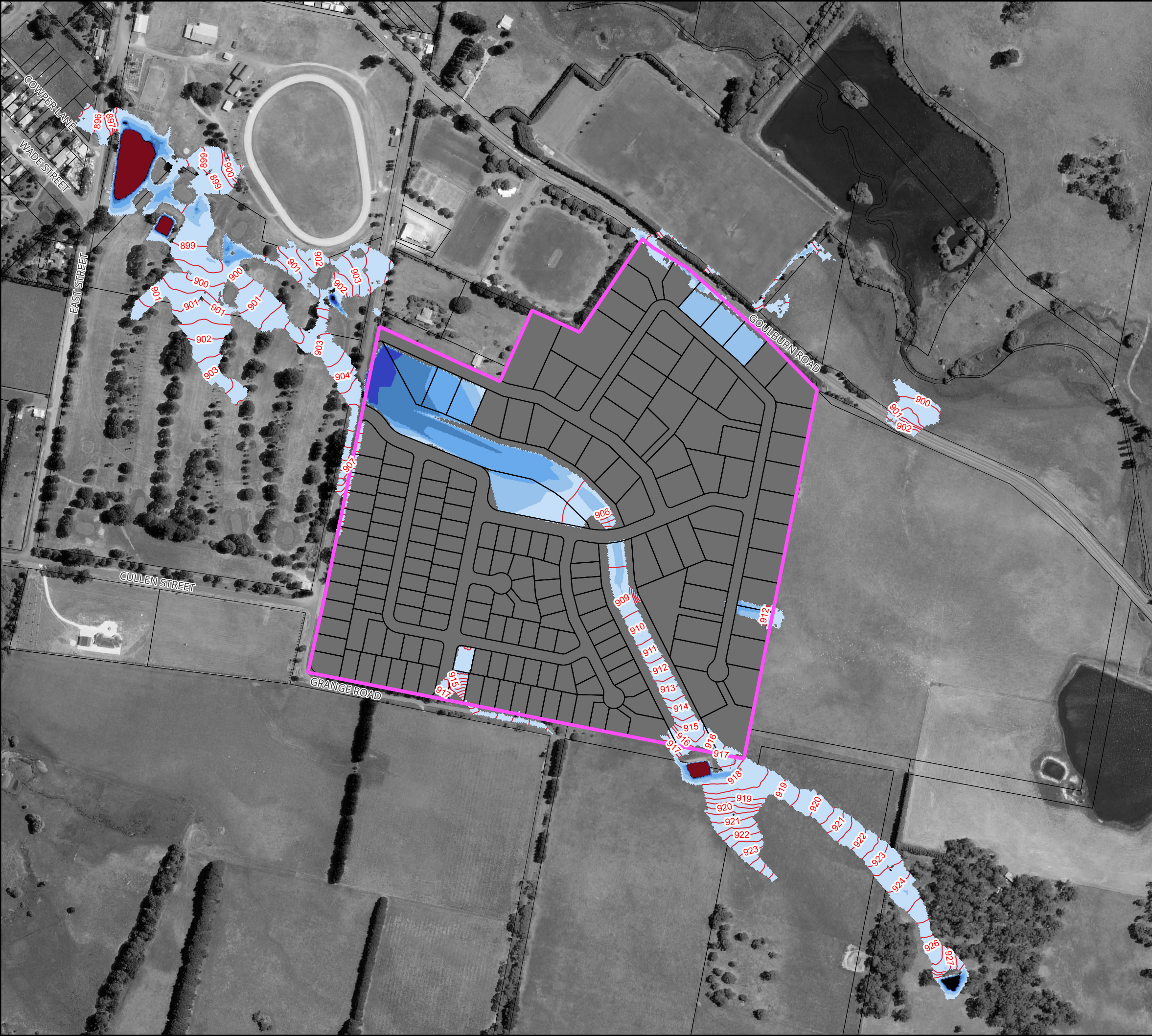
Figure 42 : Peak Floodwater Depths and Levels for the 2% AEP Flood for Proposed Conditions
