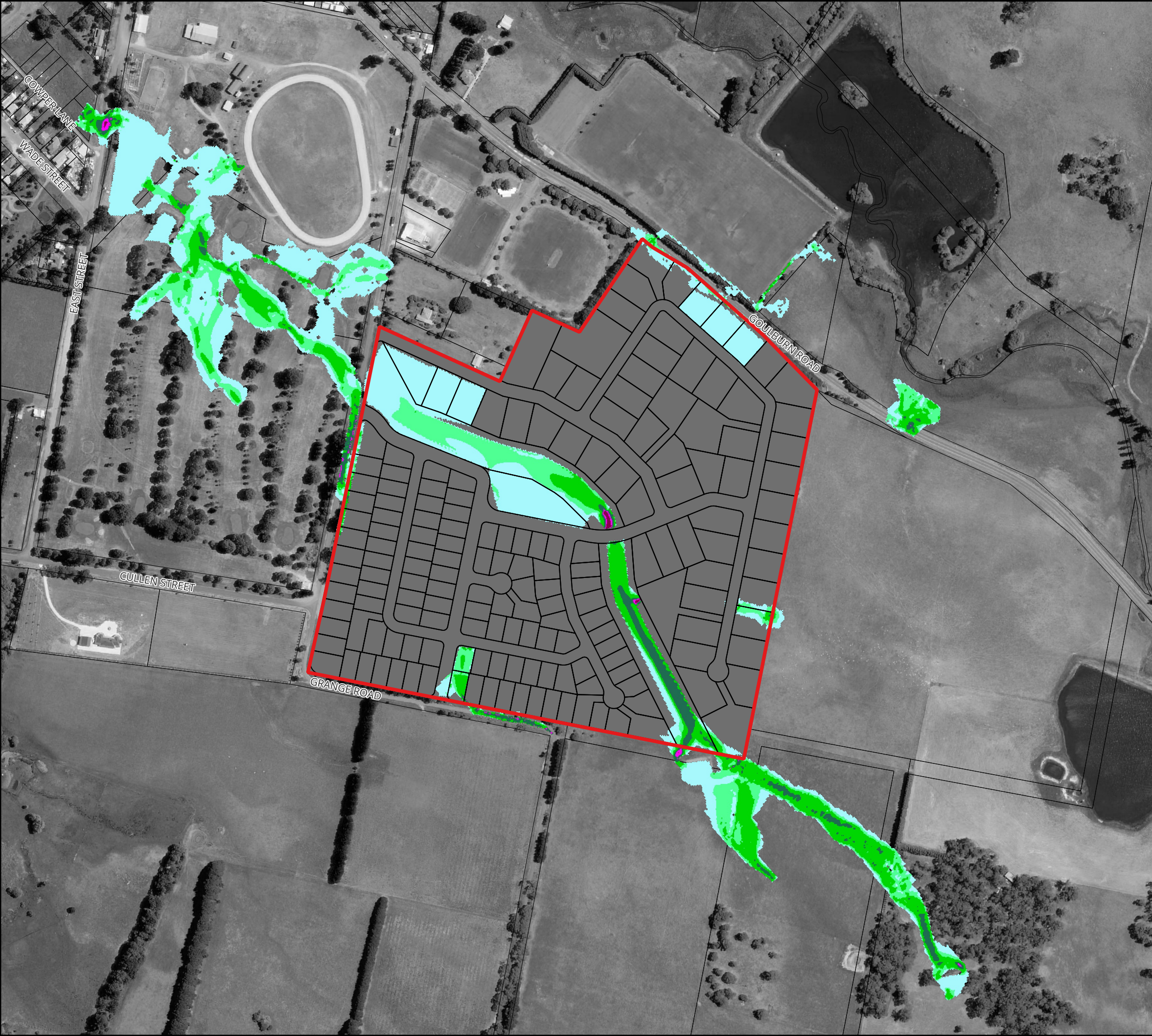
Figure 53 : Peak Flood Velocity for the 1% AEP Flood for Proposed Conditions
