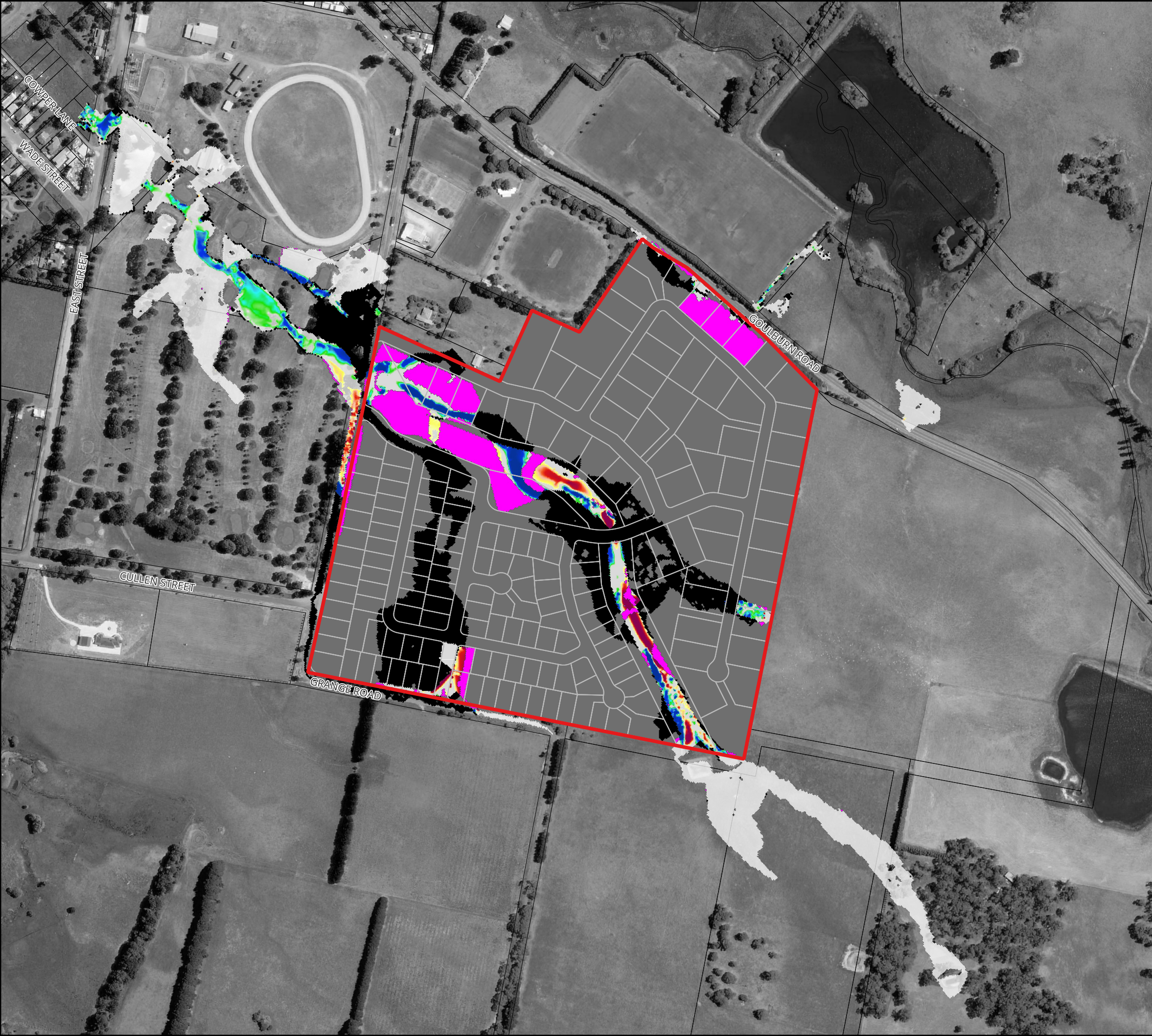
Figure 80 : Predicted Change in Peak 50% AEP Flood Velocity
